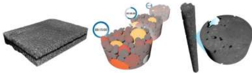
Battery cathode foil imaged at 590 nm voxel resolution
