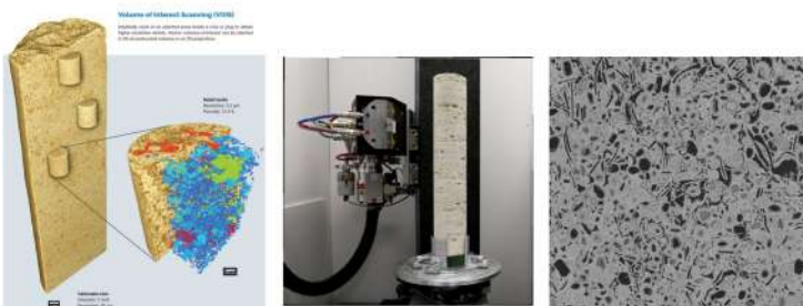
Selected volumes of interest inside a 2 inch carbonate core showing pore scale information.
