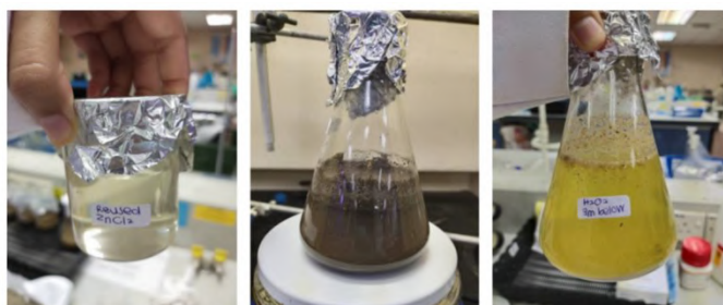
The picture above shows the ZnCl 2 solution used to extract soil samples (left), plastic waste mixed with organic matter added with oxidizing agent, H 2 O 2 then heated on a hot plate (center) and organic matter begins to decompose on day 3 of the process of plastic waste cleaning (right).
