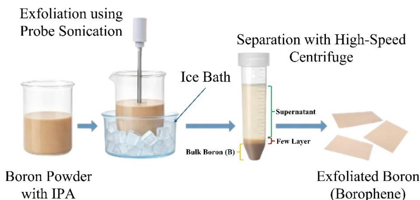
Figure 1. Schematic of the liquid-phase sonochemical exfoliation process: boron powder (B) is dispersed in IPA, treated via probe ultrasonication, and centrifuged to separate unexfoliated material from the borophene nanosheet supernatant to extract exfoliated borophene.
