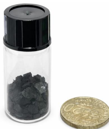
Figure 1. Macroscopic appearance of the synthesized PANI–SiO 2 nanocomposite. The blackish-green powder was stored in a sealed glass vial.
