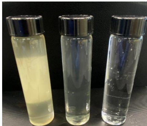
Figure 6. Effluent appearance during the core-flood sequence: initial brine (right), Tween-80 stage (middle), and final brine after scCO 2 (left).
