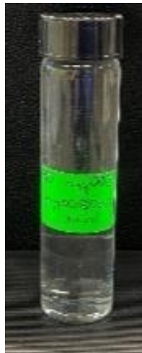
Figure 4. Turbidity observation of Tween 80(1500 ppm) in 200000 ppm brine after 24h, showing no visible precipitation or cloudiness, confirming surfactant stability.
