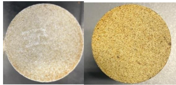
Figure 5. Inlet section views comparing the core after(left) and before(right) flooding.
