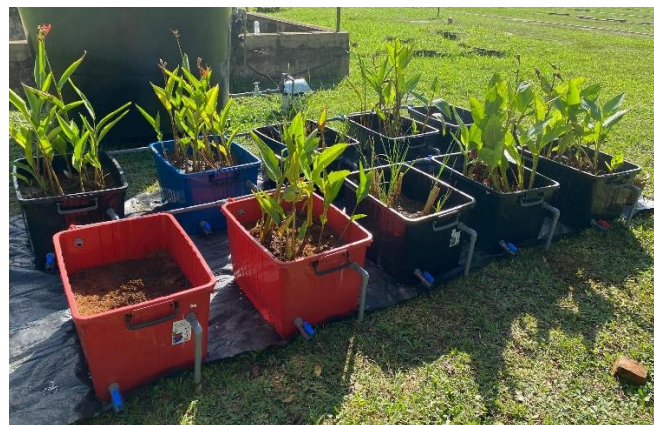
Figure 3. Design layout of the mesocosm constructed wetland setup.
