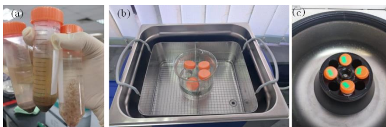
Figure 5. (a) The adsorbent was placed in a standard metal solution in a 50 mL centrifuge tube with a concentration of 1000 ppm; (b) The sample was immersed in an ultrasonic bath for 30 min at 40 kHz; (c) Sample ready for centrifuge.
