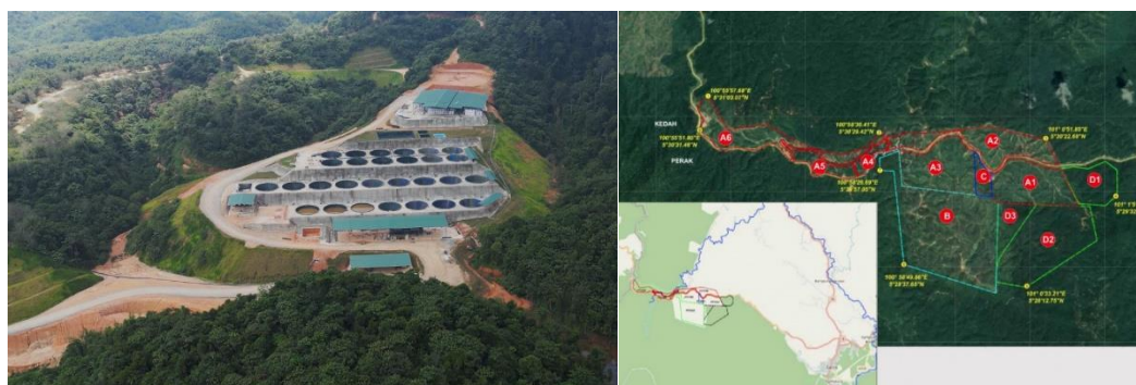
Figure 1. Aerial image and map of the REE mine at Kenering, Perak, Malaysia that adopts in-situ leaching method.
