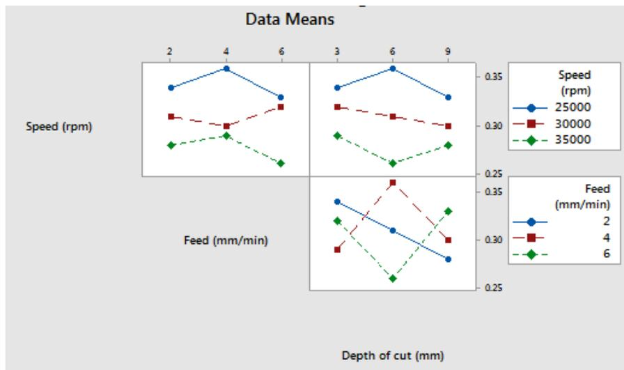
Figure 7. Interaction plot for cutting force.
