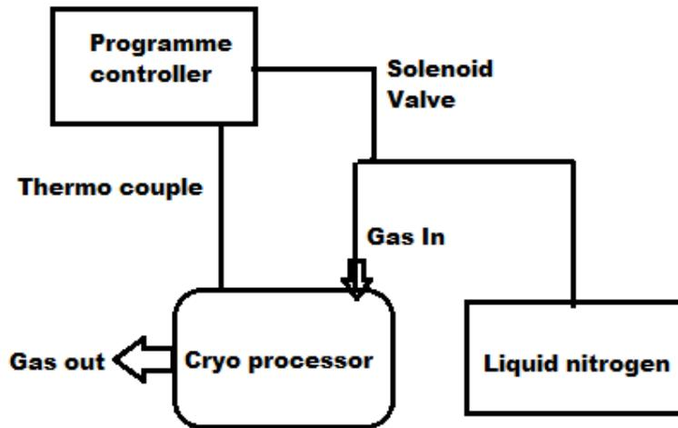
Figure 1. Line diagram of cryogenic treatment.
