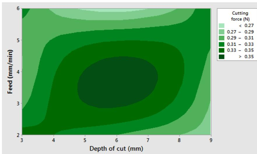
Figure 6. contour plots between depth of cut and feed.
