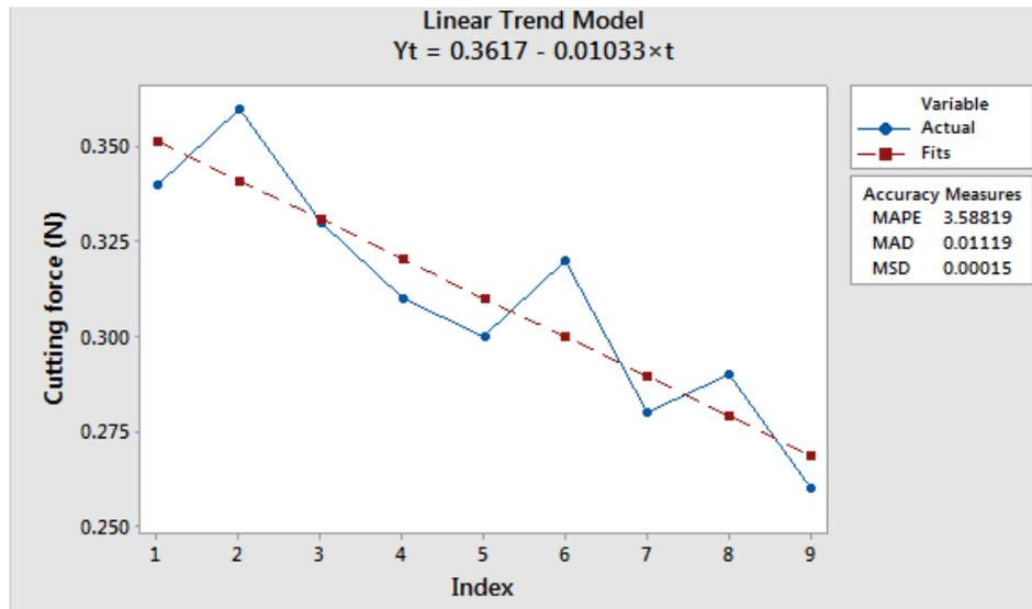
Figure 8. Trend analysis of cutting force.
