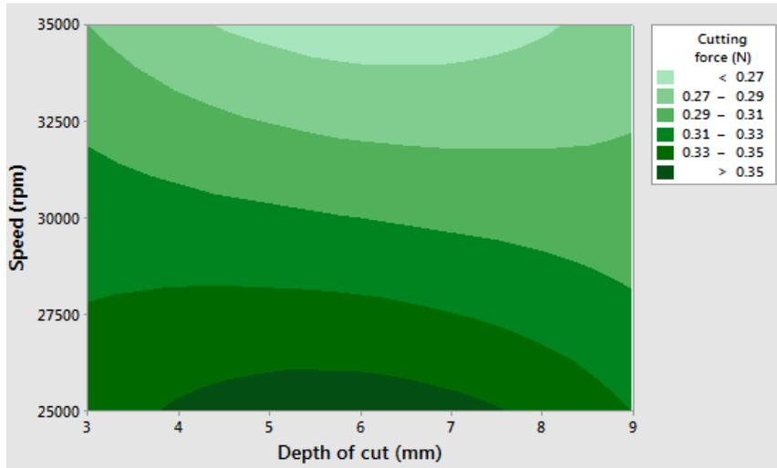
Figure 5. contour plots between depth of cut and speed
