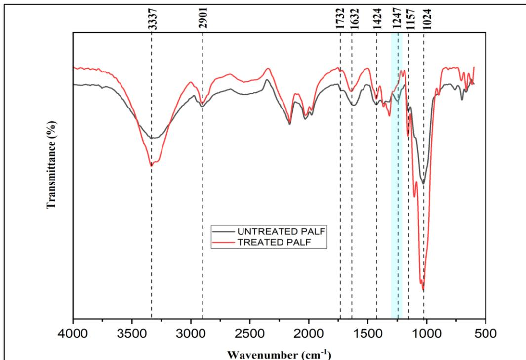
**Figure 3.** FTIR analysis of untreated and NaOH treated PALF.
