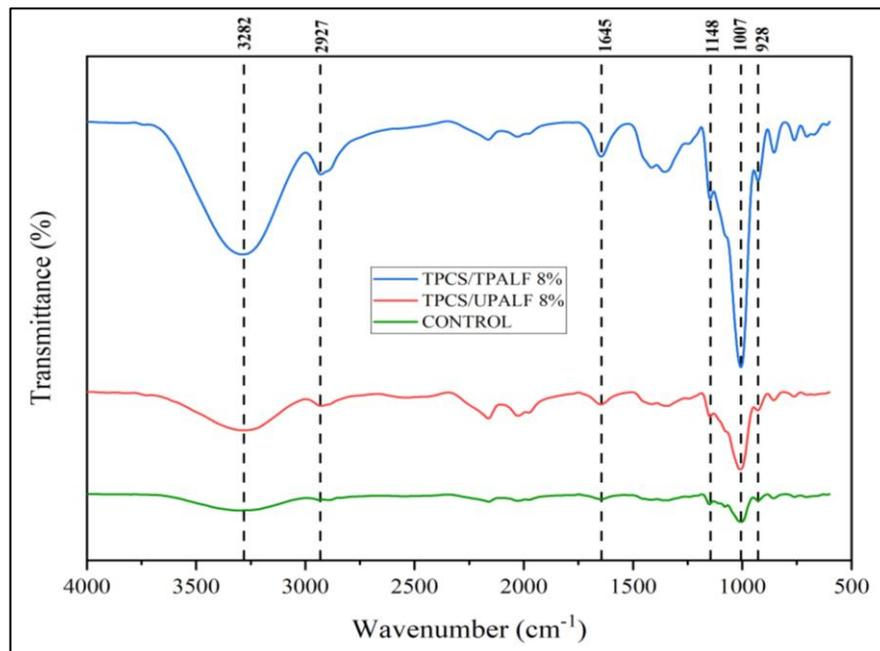
**Figure 4.** Comparison of FTIR analysis between control, untreated and treated TPCS/PALF 8% composites film.
