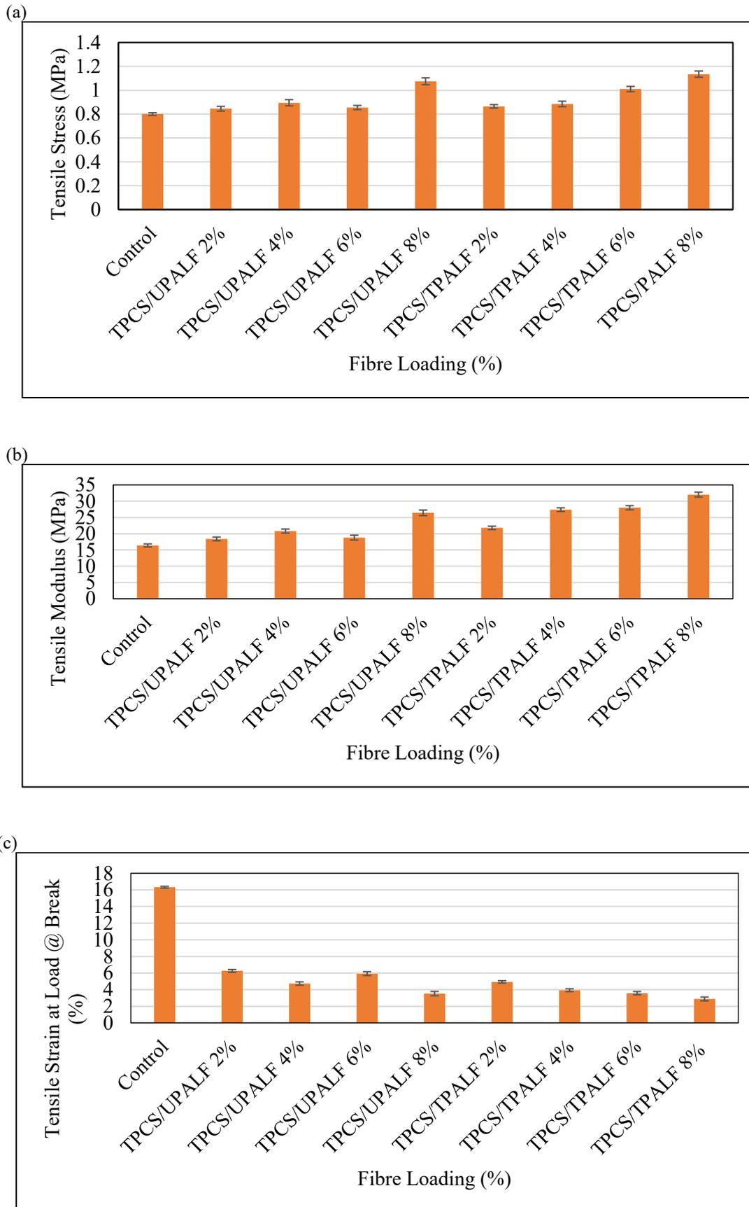
**Figure 5.** Tensile properties of the control and the thermoplastic cassava starch/PALF bioplastic at 2, 4, 6, and 8 wt % of untreated and treated: (a) tensile strength, (b) tensile modulus, and (c) elongation at break.
