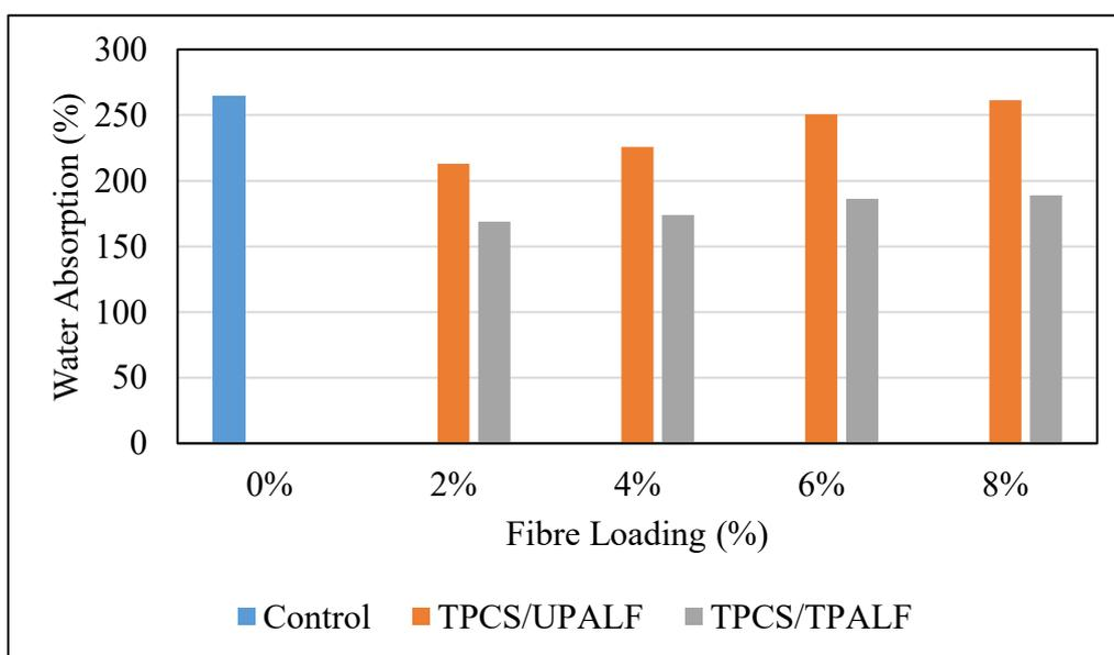
**Figure 2.** Water absorption of control, TPCS/UPALF and TPCS/TPALF composite films for 180 min time immersion.
