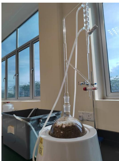
Figure 2. The apparatus setup of standard hydrodistillation for agarwood essential oil.
