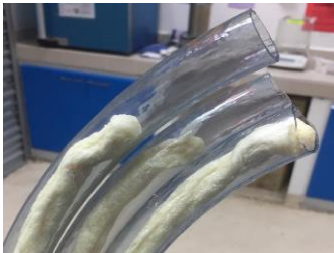
Figure 8. 3 samples of shrunken polyurethane with a ratio of 1:0.5 in the hose.
