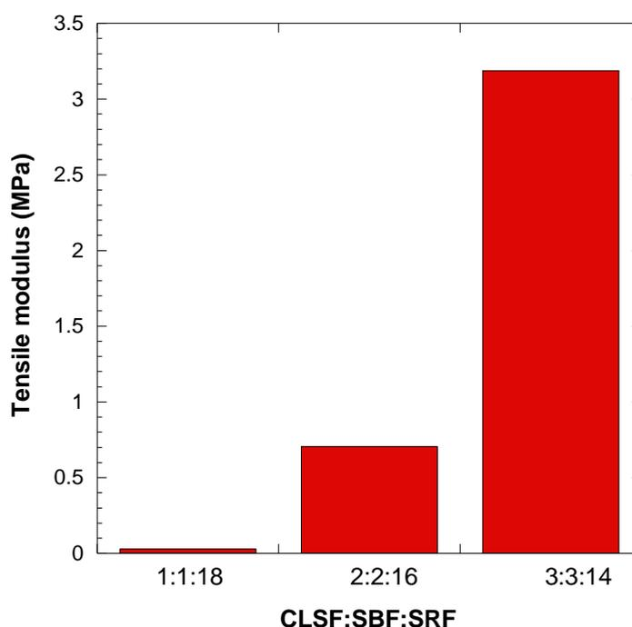
**Figure 8.** Tensile modulus (MPa) of BSB with various composition ratio of CLSF:SBF:SRF
