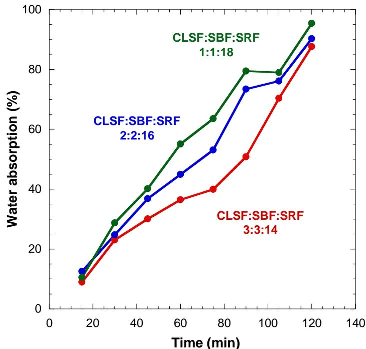
Figure 2. Water absorption (%) of BSB with various composition ratio of CLSF:SBF:SRF as a function of time (min)
