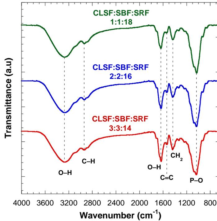
Figure 6. FTIR spectra of BSB with various composition ratio of CLSF:SBF:SRF
