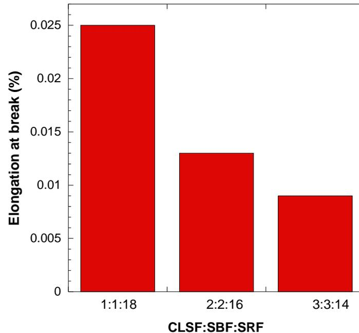
**Figure 9.** Elongation at break (%) of BSB with various composition ratio of CLSF:SBF:SRF
