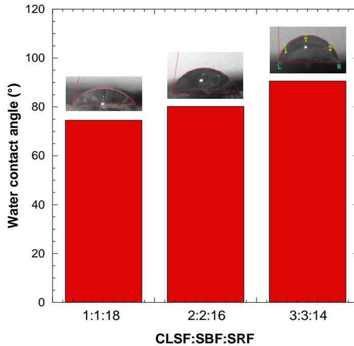
Figure 1. Water contact angle (°) of BSB with various composition ratio of CLSF:SBF:SRF
