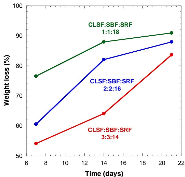
**Figure 4.** Weight loss (%) of BSB with various composition ratio of CLSF:SBF:SRF as a function of decomposition time (days)
