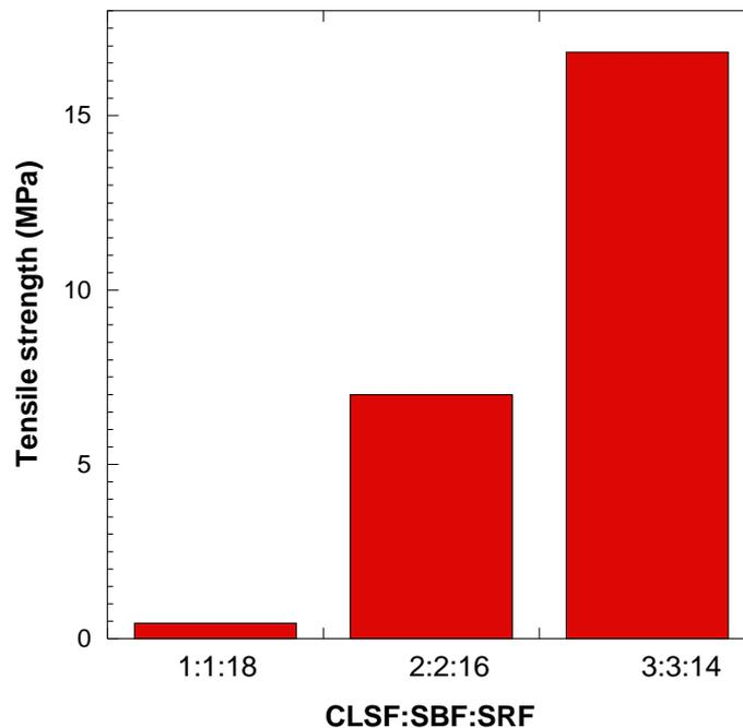
Figure 7. Tensile strength (MPa) of BSB with various composition ratio of CLSF:SBF:SRF
