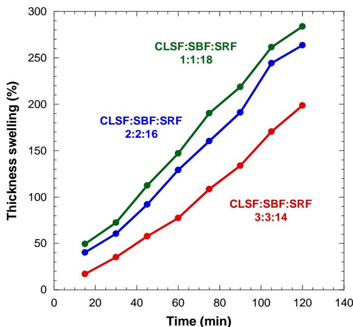
**Figure 3.** Thickness swelling (%) of BSB with various composition ratio of CLSF:SBF:SRF as a function of time (min)
