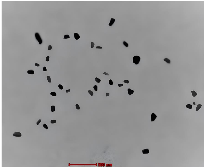
Figure 4. TEM photomicrograph of the selected formulation (lipid: 7.5% (w/w), surfactant: 3.5% (v/v) drug/lipid ratio: 1% (w/w)) of prednisolone-loaded SLNs at 11,500x magnification.
