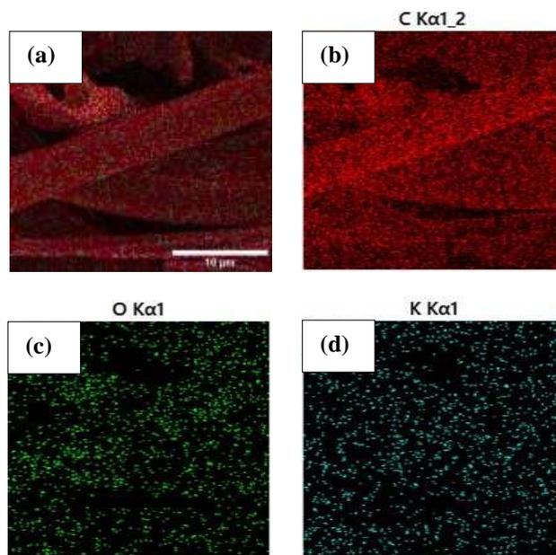
**Figure 3.** EDX analysis image of KF (a) and the related C, O and K elemental mapping images are displayed in (b), (c) and (d) respectively.
