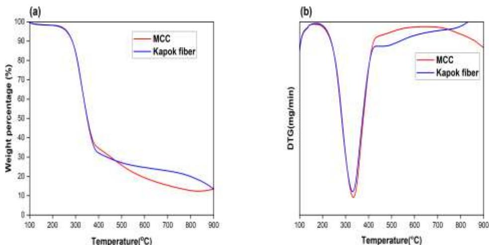
Figure 7. (a) TGA curves, and (b) DTG curves for the kapok fibre and MCC samples.
