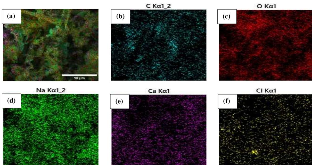
**Figure 4.** EDX analysis image of MCC (a) and the related C, O, Na, Ca and Cl elemental mapping images are displayed in (b), (c), (d), (e) and (f) respectively.
