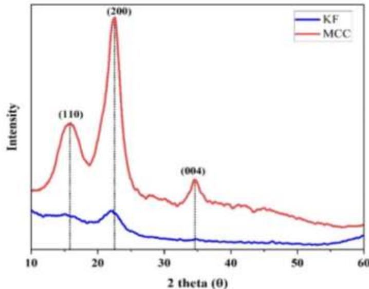
**Figure 8.** XRD diffraction patterns of KF and MCC
