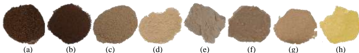
Figure 2. Cocoa shell powder samples: (a) RM (b) GM (c) HA5 (d) HA17.5 (e) CAM17.5 (f) CA17.5 (g) SA17.5 (h) NA17.5.
