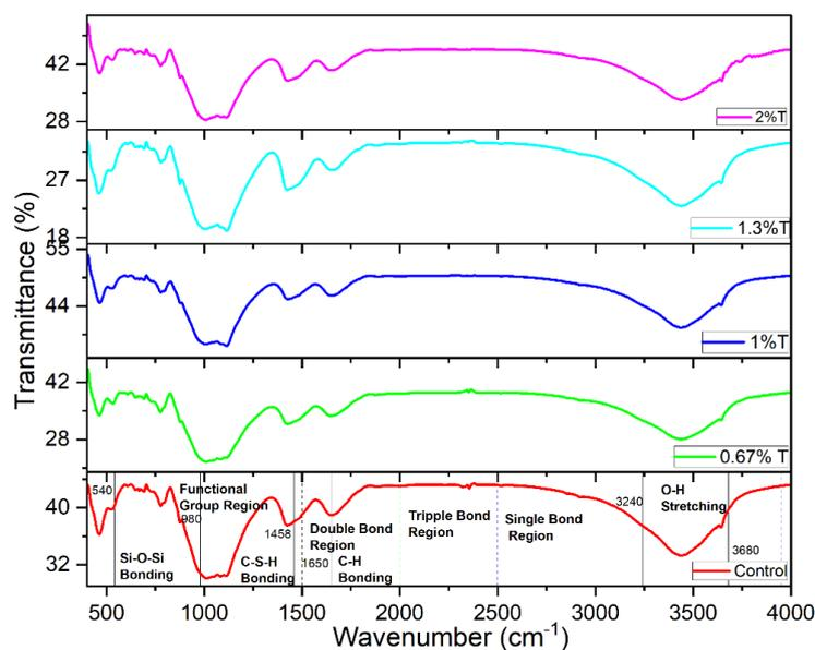
Figure 2. FTIR spectra of HPC with varying content of TiO<sub>2</sub>.
