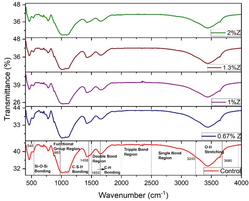
Figure 3. FTIR spectra of HPC with varying content of ZnO.
