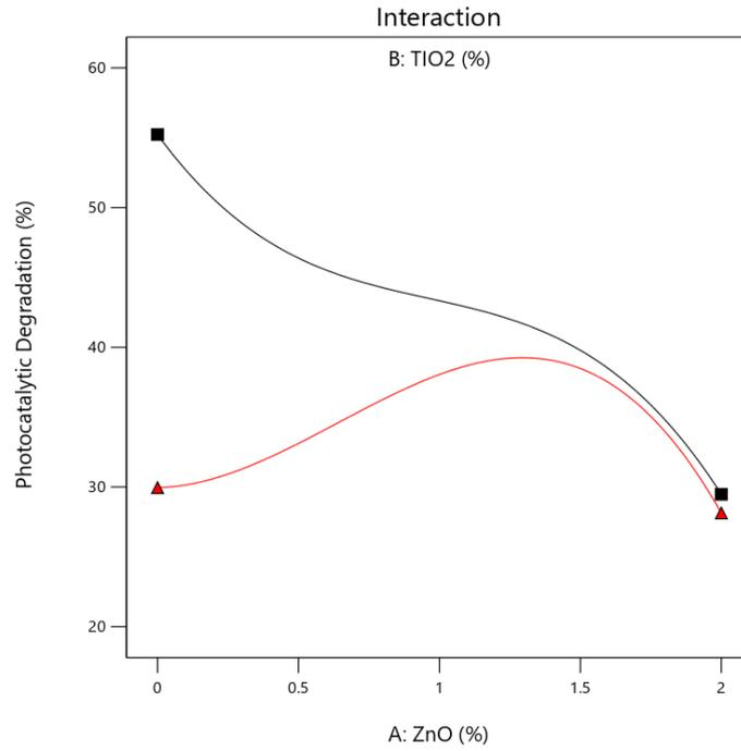
Figure 6. Interactive effect of TiO<sub>2</sub> and ZnO on PD.
