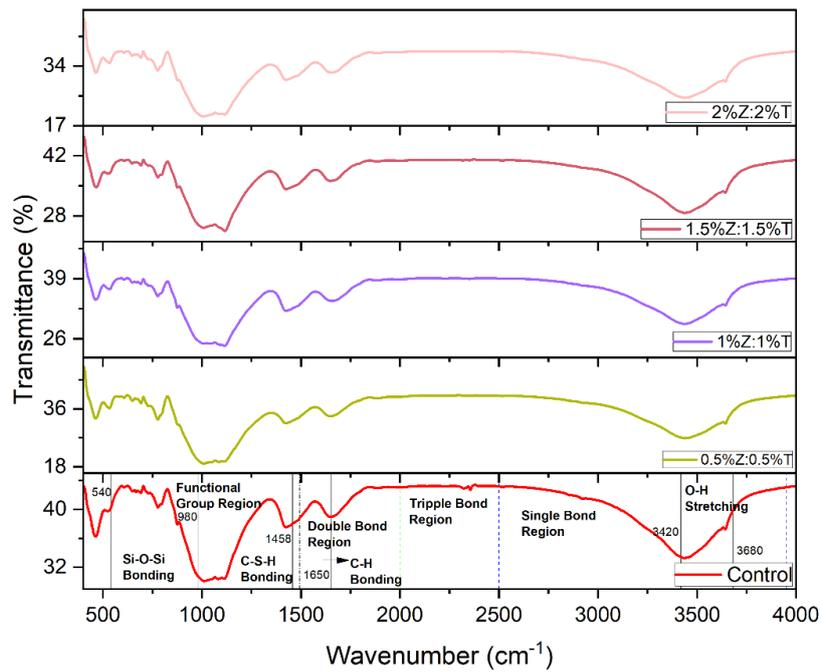
Figure 4. FTIR spectra of HPC with equal combinations of TiO<sub>2</sub> and ZnO contents.
