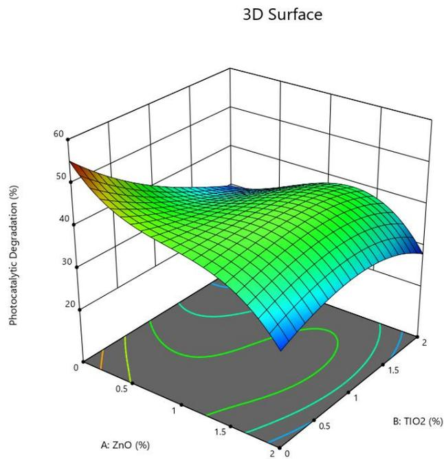
Figure 7. 3D surface plot of the effect of TiO<sub>2</sub> and ZnO on PD.
