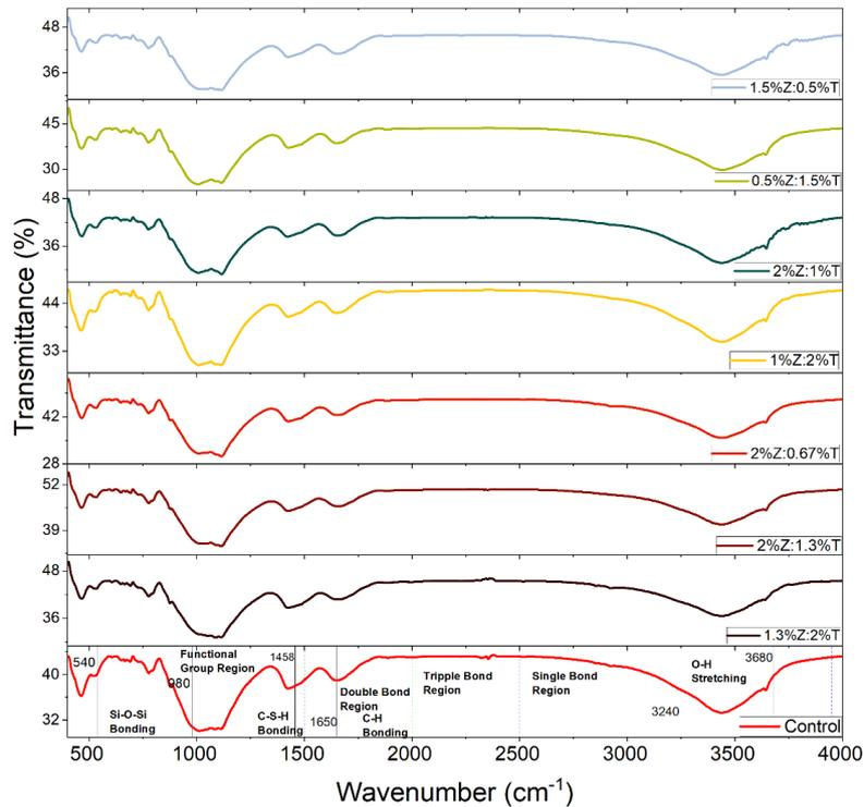
Figure 5. FTIR spectra of HPC with varied combinations of  $\text{TiO}_2$  and  $\text{ZnO}$  contents.
