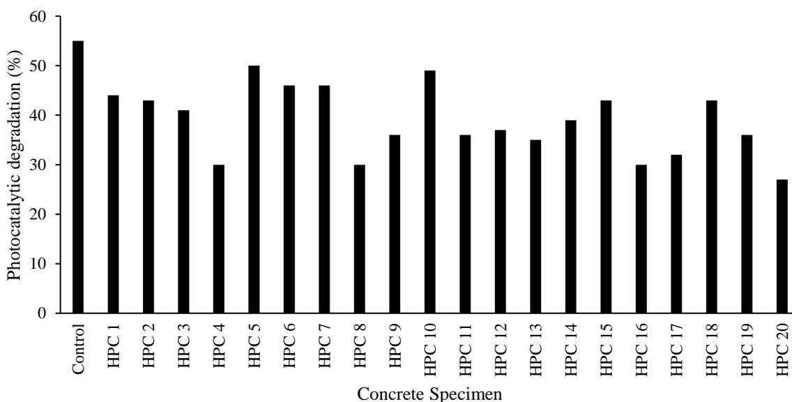
**Figure 1.** Photocatalytic degradation (PD) of concrete samples with TiO<sub>2</sub> and ZnO after 100 hrs of UV irradiation.
