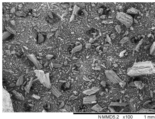
Figure 3. SEM of the BCP at 100× magnification.
