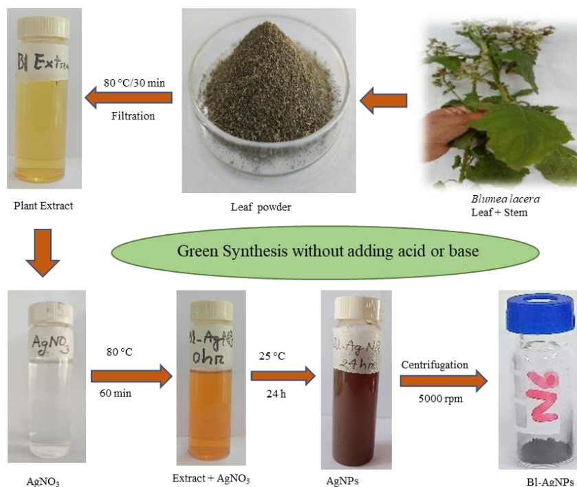
Figure 1. Schematic illustration of the synthesis of BI-AgNPs .
