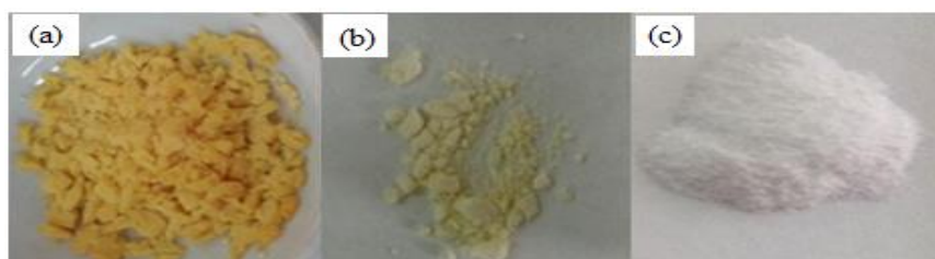
Figure 2. Synthesis Result of MIPs and NIPs: (a) MIPs Before Leaching, (b) MIPs After Leaching, and (c) NIPs.
