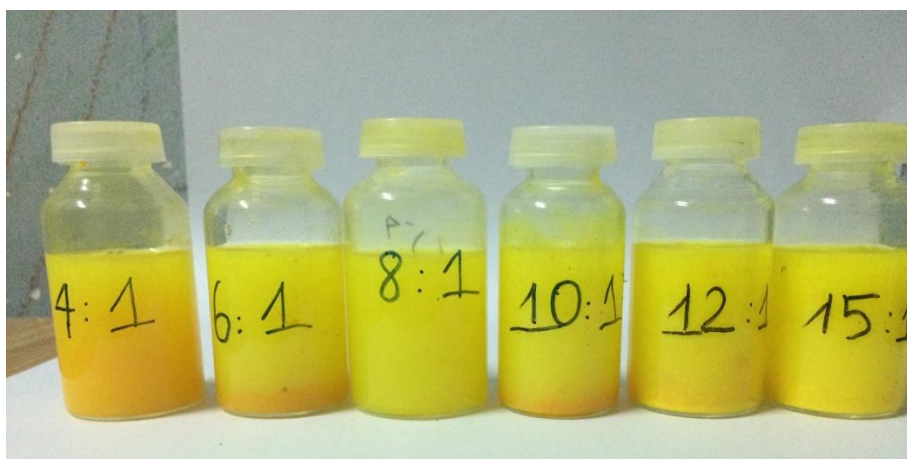
Figure 1. Image of micellar formulations with mass ratios of mPEC to curcumin of 4:1 to 15:1 (left to right).
