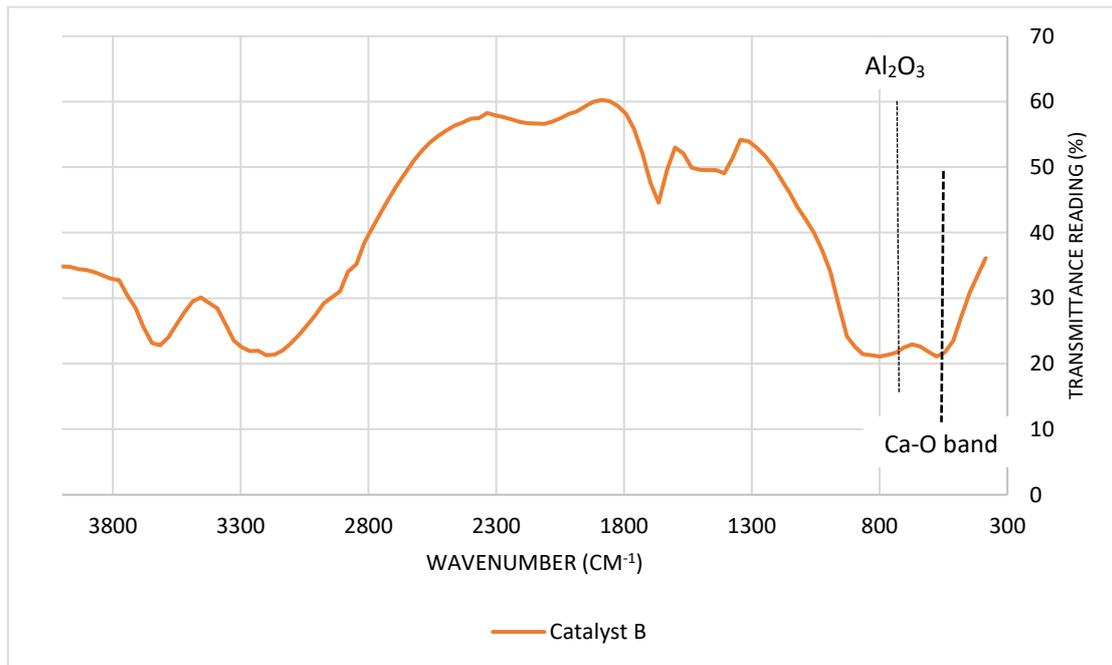
**Figure 2.** FTIR-KBr spectrum of CaO/FeO/Al<sub>2</sub>O<sub>3</sub> (Catalyst B).
