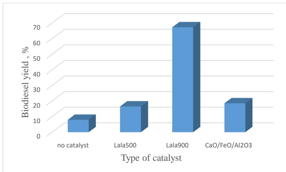
Figure 9. Effect of type of catalyst for biodiesel production.
