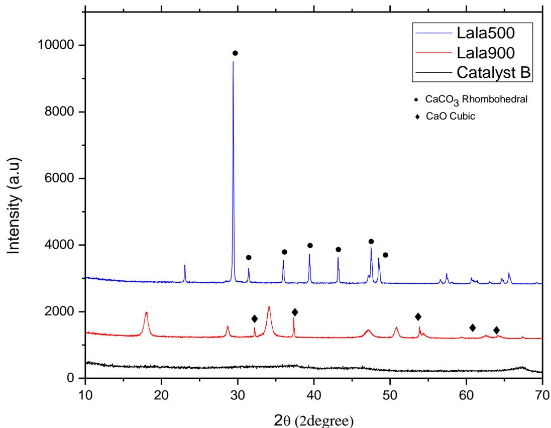
**Figure 5.** XRD diffractogram of catalyst CaO/FeO/Al<sub>2</sub>O<sub>3</sub> (Catalyst B), clamshell calcined at 500°C (Lala50) and clamshell calcined at 900°C (Lala900).
