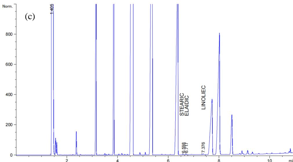
**Figure 10.** Characterization of biodiesel using gas chromatography-flame ion detector (GC-FID) for (a) CaO/FeO/Al<sub>2</sub>O<sub>3</sub> (Catalyst B), (b) clamshell calcined at 500°C (Lala500) and (c) clamshell calcined at 900°C (Lala900).
