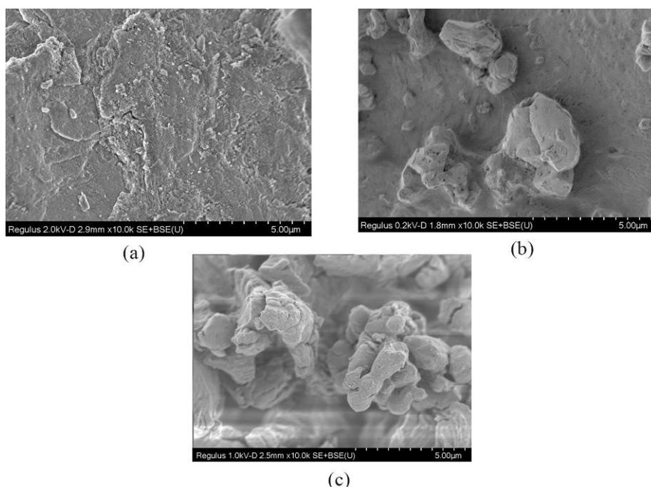
**Figure 4.** FESEM micrographs of catalysts: (a) CaO/FeO/Al<sub>2</sub>O<sub>3</sub> (Catalyst B); (b) clamshell calcined at 500°C (Lala500); and (c) clamshell calcined at 900°C (Lala900); at 10 000× magnification
