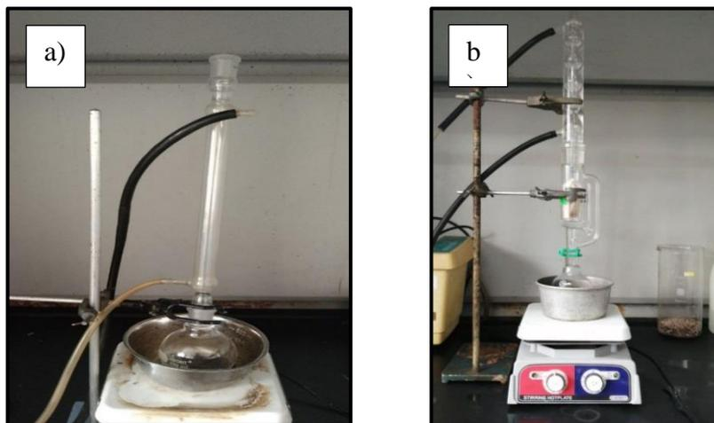
**Figure 1.** Experimental setups for: (a) In Situ Extraction; and (b) Soxhlet Extraction
