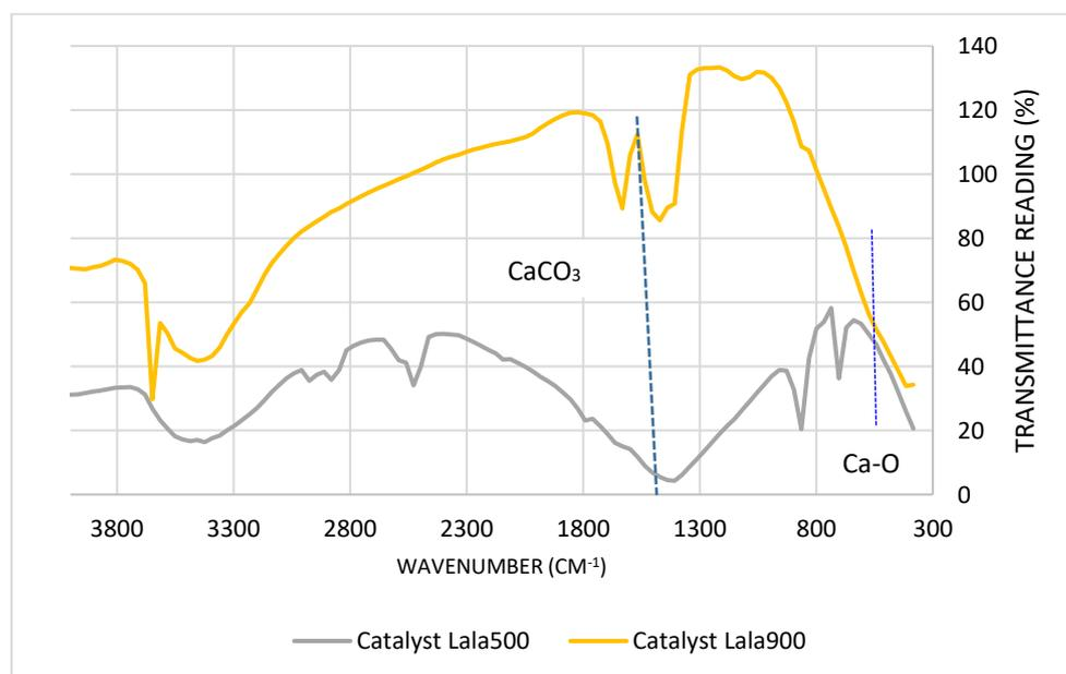
**Figure 3.** FTIR-KBr spectra of clamshell calcined at 500°C (Lala500) and at 900°C (Lala900).
