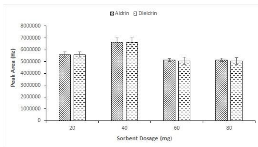
Figure 7. The effect of sorbent dosage on the DSPE method for extraction of OCPs
