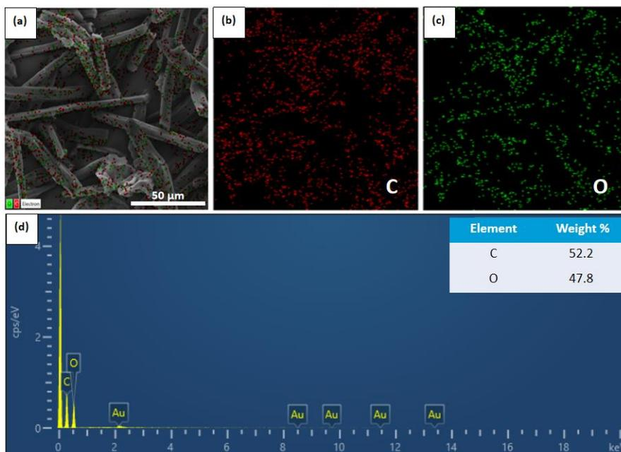
**Figure 4.** EDX analysis of (a) selected image of MCC-2 with corresponding elemental mapping images for C and O are presented in (b) and (c), respectively and (d) the elemental spectra and composition of the sample.
