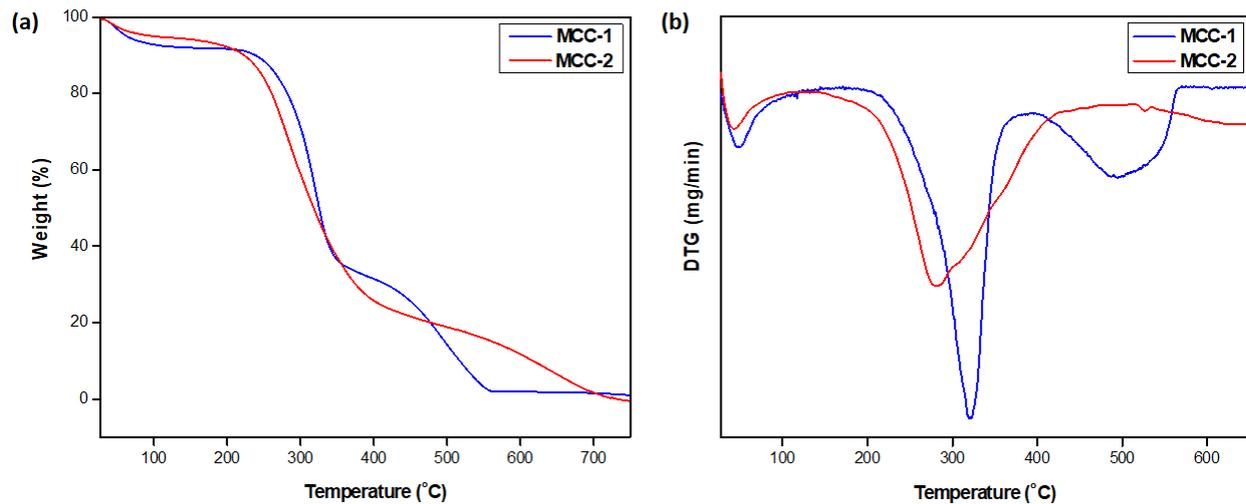
Figure 7. (a) TGA and (b) DTG curves of MCC-1 and MCC-2.
