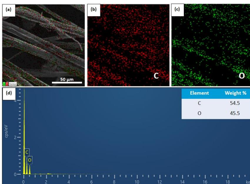
**Figure 3.** EDX analysis of (a) selected image of MCC-1 with corresponding elemental mapping images for C and O are presented in (b) and (c), respectively and (d) the elemental spectra and composition of the sample.
