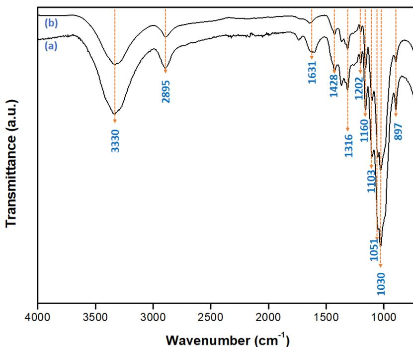
**Figure 5.** FTIR spectra of (a) MCC-1 and (b) MCC-2.
