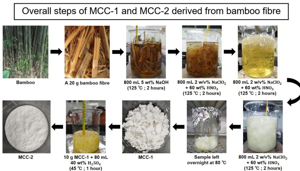
**Figure 1.** Overview of MCC-1 and MCC-2 experimental procedure.
