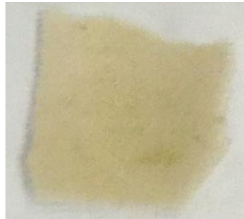
Figure 2. Condition of the fabric after 24 hours of immersion in tap water.
