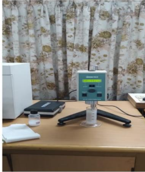
Figure 11. VC measurement of hybrid nanofluids.
