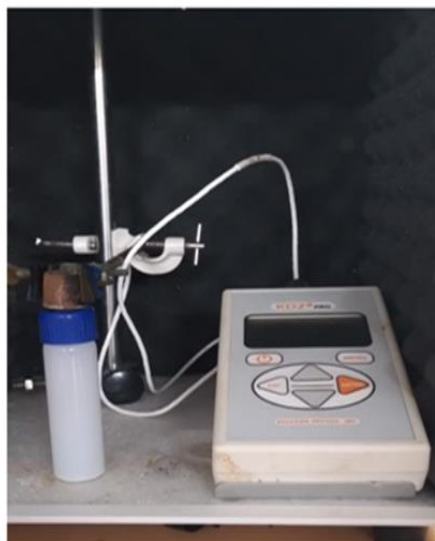
Figure 10. TC measurement of hybrid nanofluids.
