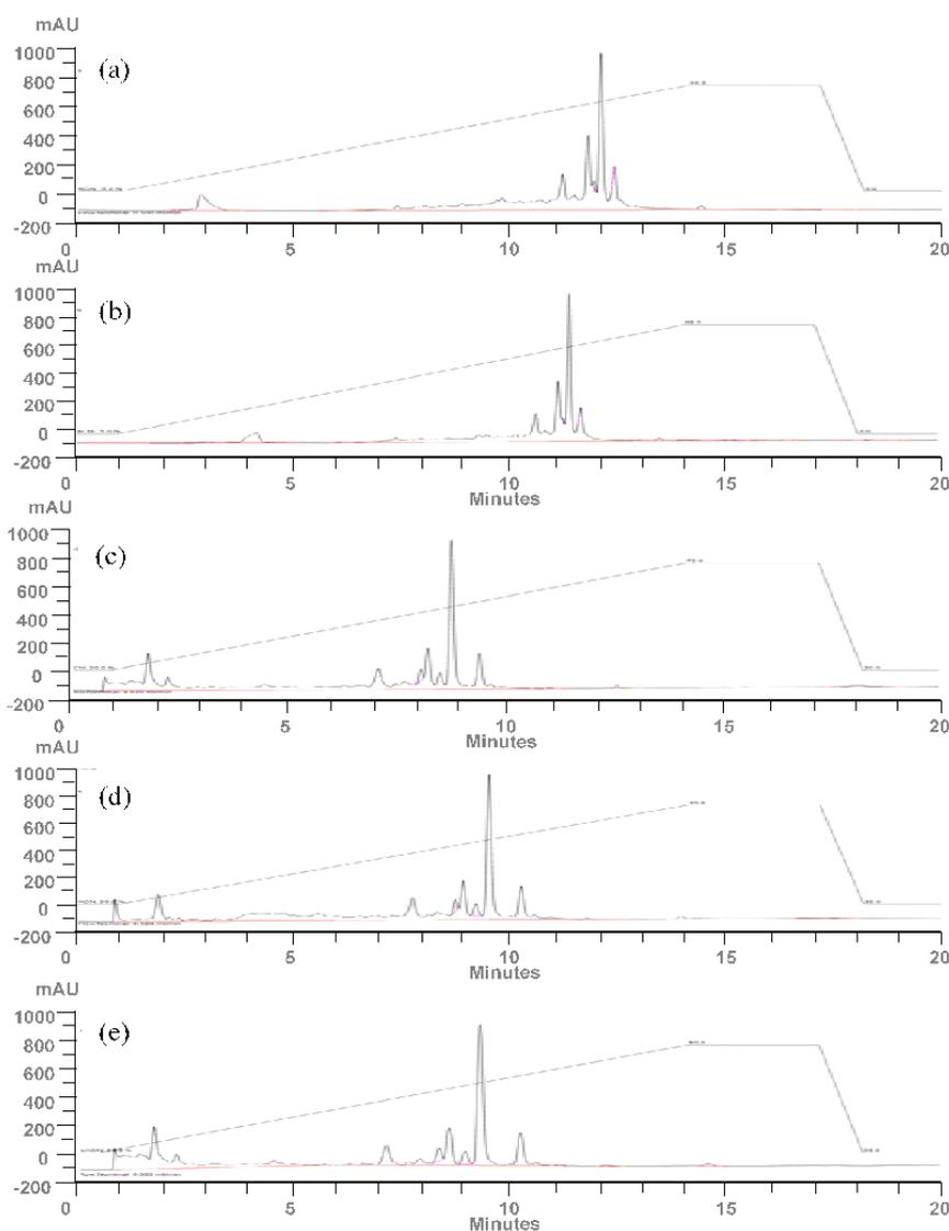
**Figure 1.** Chromatograms of stem extract on UHPLC; (a) ACN: $\text{H}_2\text{O}$  (5:95 to 95:5), (b) ACN: $\text{H}_2\text{O}$  (5:95 to 85:15), (c) ACN: $\text{H}_2\text{O}$  (20:80 to 95:5), (d) ACN: $\text{H}_2\text{O}$  (15:85 to 95:5), (e) ACN: $\text{H}_2\text{O}$  (15:85 to 85:15) in 14 minutes. The series of profiles show adjustment of solvent composition and improvement of peak resolution as well as decreasing elution time.
