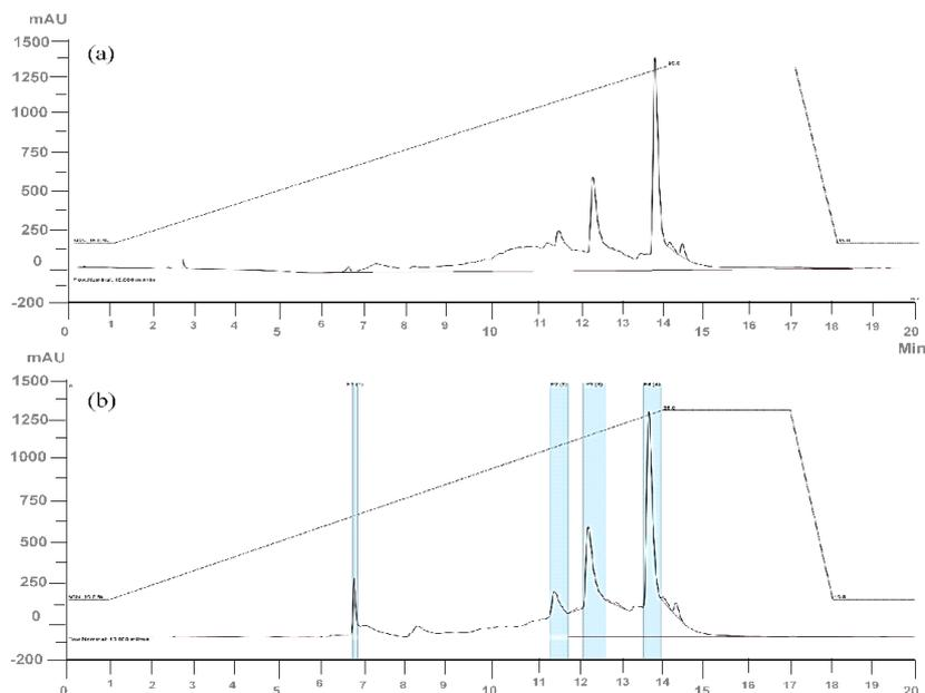
**Figure 3.** Chromatogram of leaves extract when up scaled to; (a) semi-preparative and (b) collection of its constituents, both at ACN: H<sub>2</sub>O (20:80 to 95:5) in 14 minutes.
