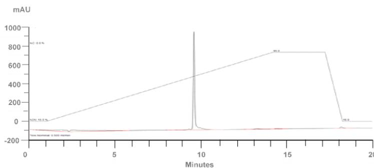
**Figure 4.** Chromatogram of a single peak, anticipated of a pure compound.
