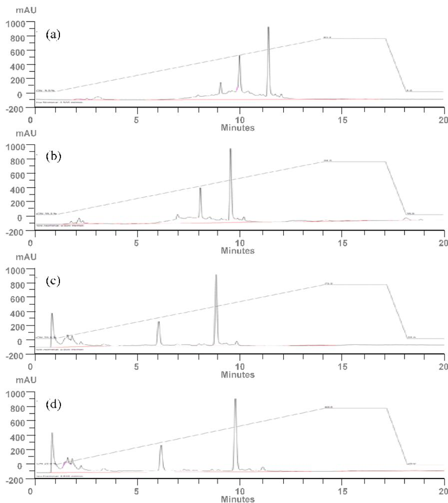
**Figure 2.** Chromatogram of leaves extract on UHPLC; (a) ACN:H<sub>2</sub>O (5:95 to 95:5), (b) ACN:H<sub>2</sub>O (5:95 to 85:15), (c) ACN:H<sub>2</sub>O (20:80 to 95:5), (d) ACN:H<sub>2</sub>O (15:85 to 95:5) in 14 minutes. The series of profiles show adjustment of solvent composition and improvement of peak resolution.
