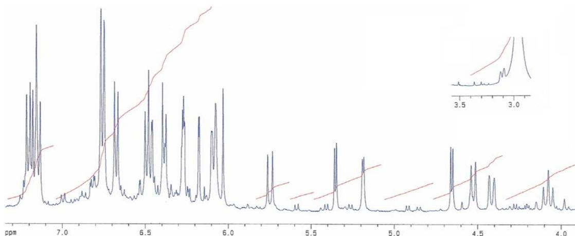
**Figure 5.**  $^1\text{H-NMR}$  of isolated compound. The experiment was run at 600 MHz in *d*-acetone.
