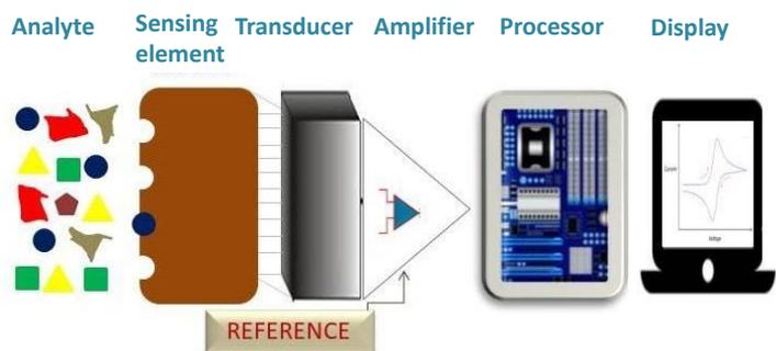
**Figure 1.** Schematic diagram of the biosensor working principles.
