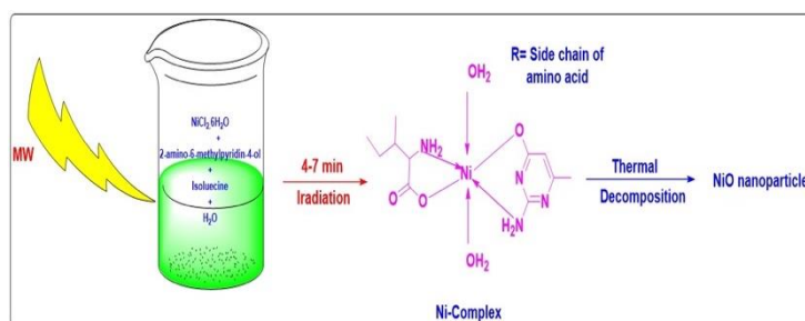
Figure 1. Schematic Representation of the Preparation of Ni(II) Complex and NiO Nanoparticles
