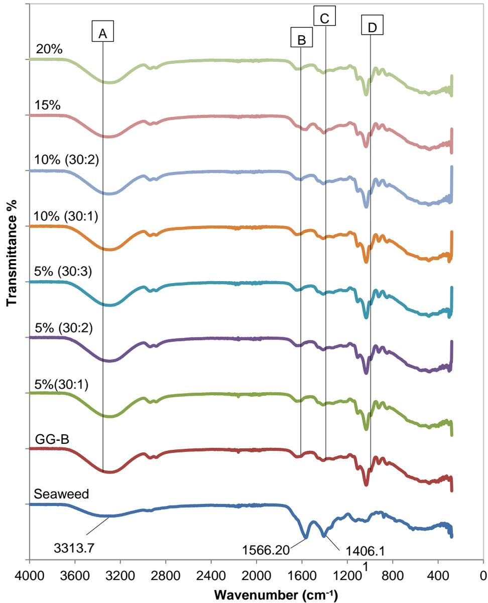
**Figure 1.** FTIR spectra of seaweed, gellan gum beads (GG-B), and GG-SB at different concentrations (5%, 10%, 15% and 20% w/v).
