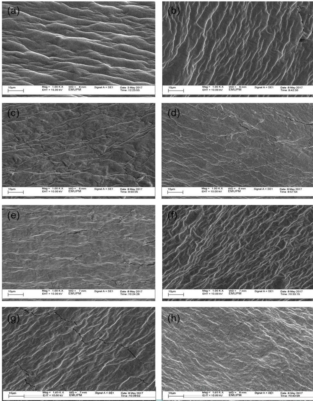
**Figure 3.** Cross-sectional morphology (1000x magnification) of (a) GG-B, (b) 5% GG-SB (30:1), (c) 5% GG-SB (30:2), (d) 5% GG-SB (30:3), (e) 10% GG-SB (30:1), (f) 10% GG-SB (30:2), (g) 15% GG-SB (30:1), (h) 20% GG-SB (30:1).
