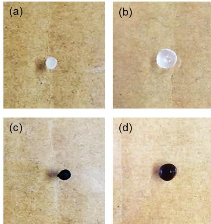
**Figure 5.** A gellan gum bead, GG-B (a) before immersion, (b) after immersion, and a gellan gum bead loaded with seaweed, GG-SB (c) before immersion, and (d) after immersion in the pH 7 solution.
