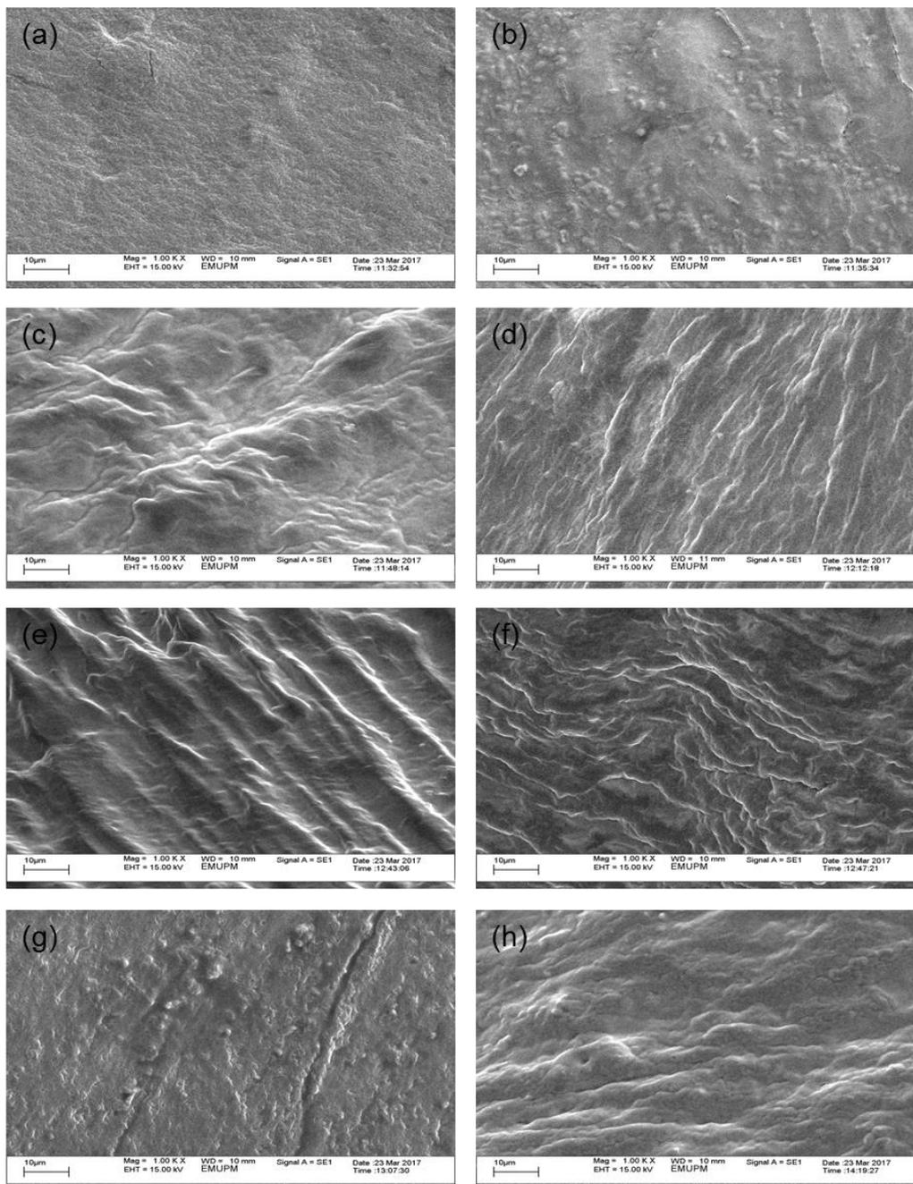
**Figure 2.** Surface morphology (1000x magnification) of (a) GG-B, (b) 5% GG-SB (30:1), (c) 5% GG-SB (30:2), (d) 5% GG-SB (30:3), (e) 10% GG-SB (30:1), (f) 10% GG-SB (30:2), (g) 15% GG-SB (30:1), (h) 20% GG-SB (30:1).
