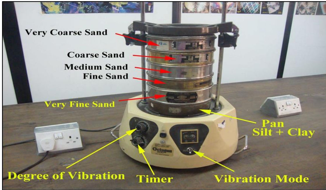
Figure 1. Sieves used for volumetric analysis with a vibrating device.
