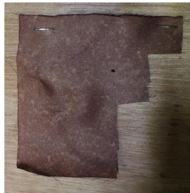
Figure 1. The condition of the fabric after 7 days of exposure in an abandoned building
