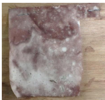
Figure 2. Condition of the fabric after 7 days of exposure to the outdoor jungle area
