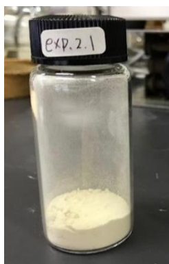
Figure 2. The off-white precipitate of the product produced at 110°C
