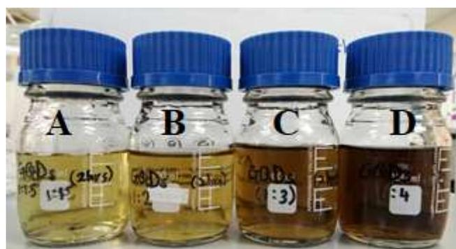
**Figure 2.** Digital image of the GQDs samples produced using various NaOH concentrations (a) GQD1, (b) GQD2, (c) GQD3 and (d) GQD4.
