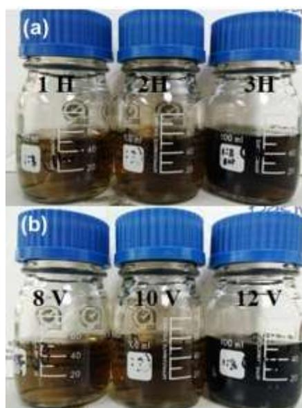
**Figure 3.** Digital images of GQDs samples produced (a) under different reaction time of 1 H (GQD5), 2 H (GQD3) and 3 H (GQD6), and (b) under different voltage of 8 V (GQD7), 10 V (GQD3) and 12 V (GQD8).
