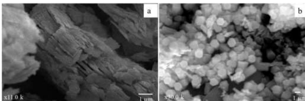
**Figure 3.** SEM images of a) kaolin precursor and b) kalsilite synthesized at 190 °C using 0.75 M KOH
