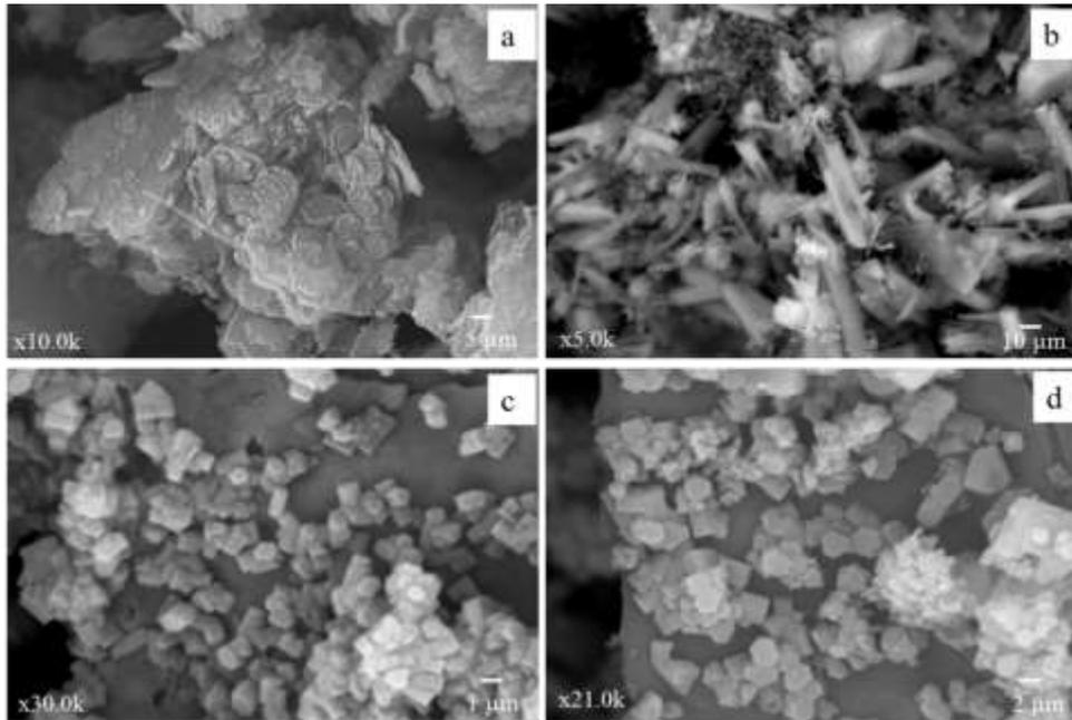
**Figure 4.** SEM images of the products after treatment with a) 0.25 M KOH, b) 0.50 M KOH, c) 0.75 M KOH and d) 1.0 M KOH at 190 °C.
