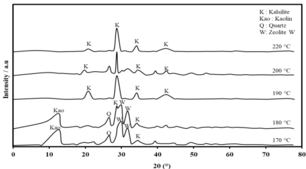
**Figure 2.** XRD diffractograms of hydrothermal reaction products obtained with 0.75 M KOH at various reaction temperatures.
