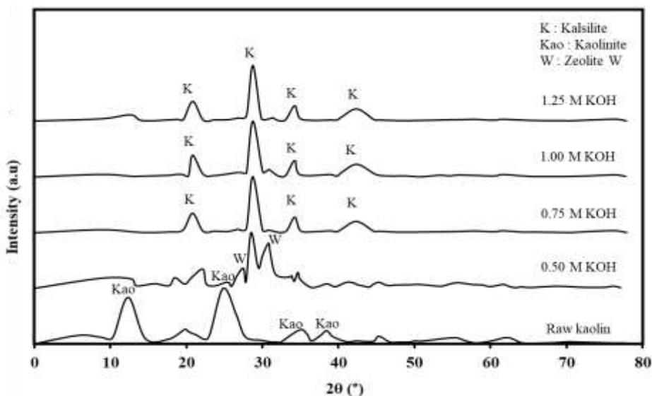
**Figure 1.** XRD diffractograms of hydrothermal reaction products obtained with various KOH concentrations at 190 °C.
