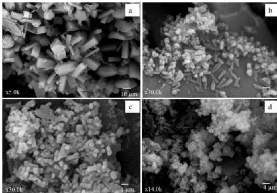
**Figure 5.** SEM images of the products obtained when treated with 0.75 M KOH at different temperatures a) 170 °C, b) 180 °C, c) 190 °C and d) 200 °C .
