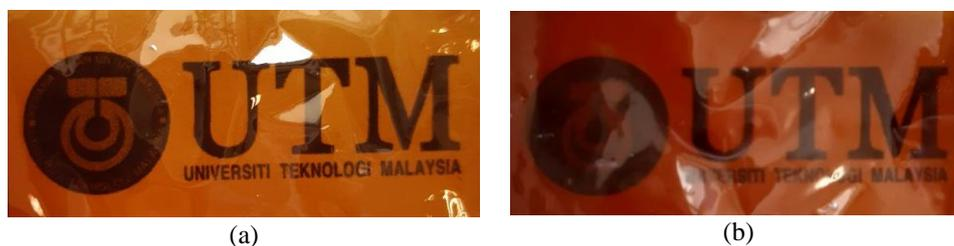
**Figure 2.** Photographic images of membranes (a) PBI/Fc-1 and (b) PBI/Fc-5
