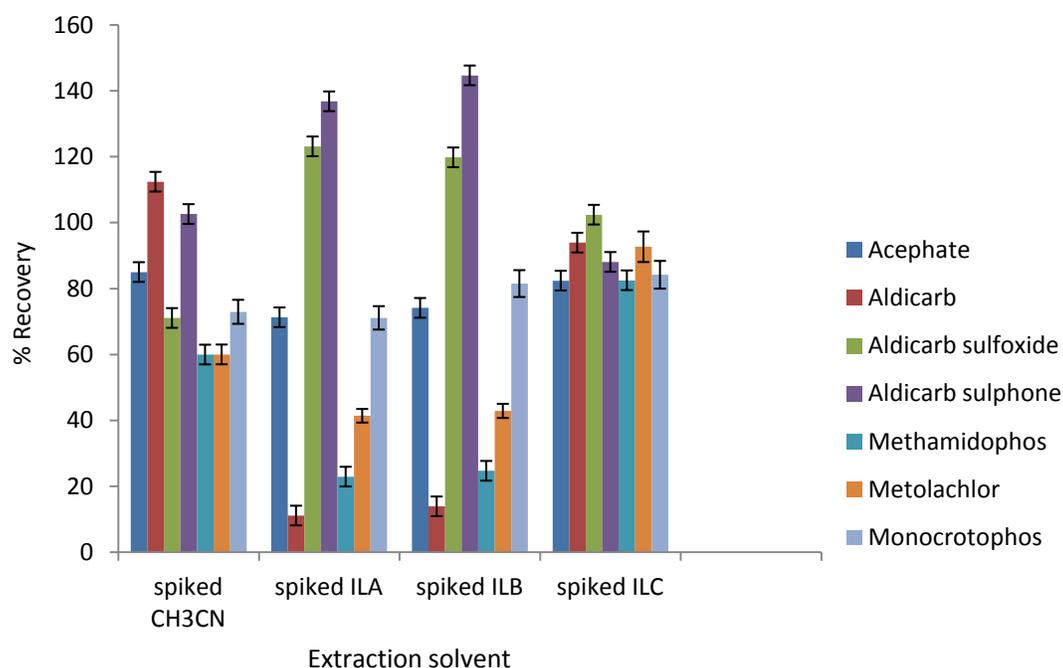
**Figure 4.** Comparison of spiked acetonitrile and the three ionic liquids neat reagents (n = 3). Error bars represent the standard deviation.
