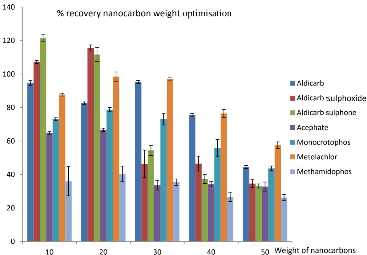
**Figure 6.** Evaluating effect of varying the weights of nanocarbons on spiked samples on sample clean-up (n = 3). Error bars represent the standard deviation.
