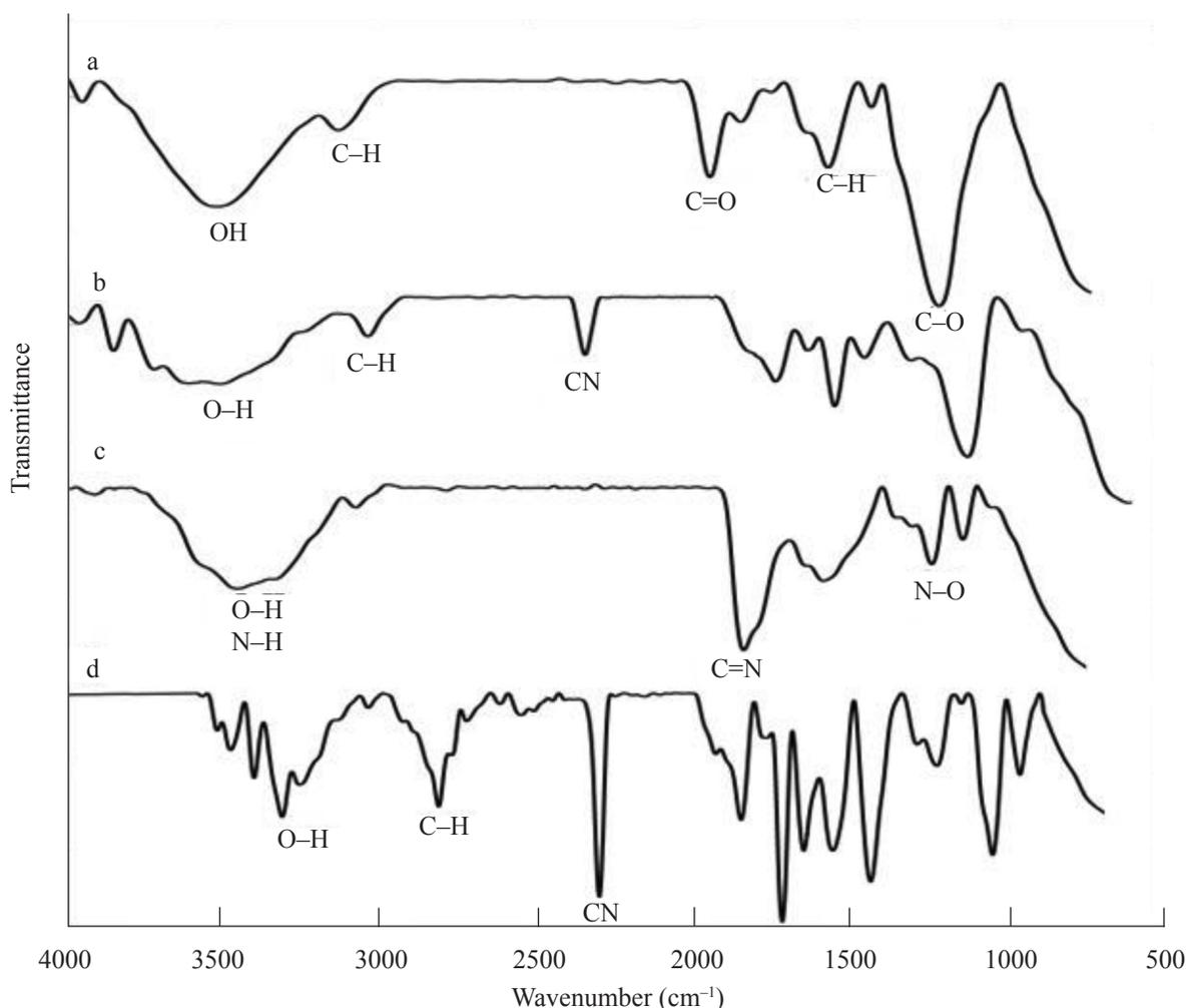
**Figure 1.** IR spectra of (a) CS (b) poly(AN-g-CS) (c) amidoxime-modified poly(AN-g-CS) and (d) homoPAN.
