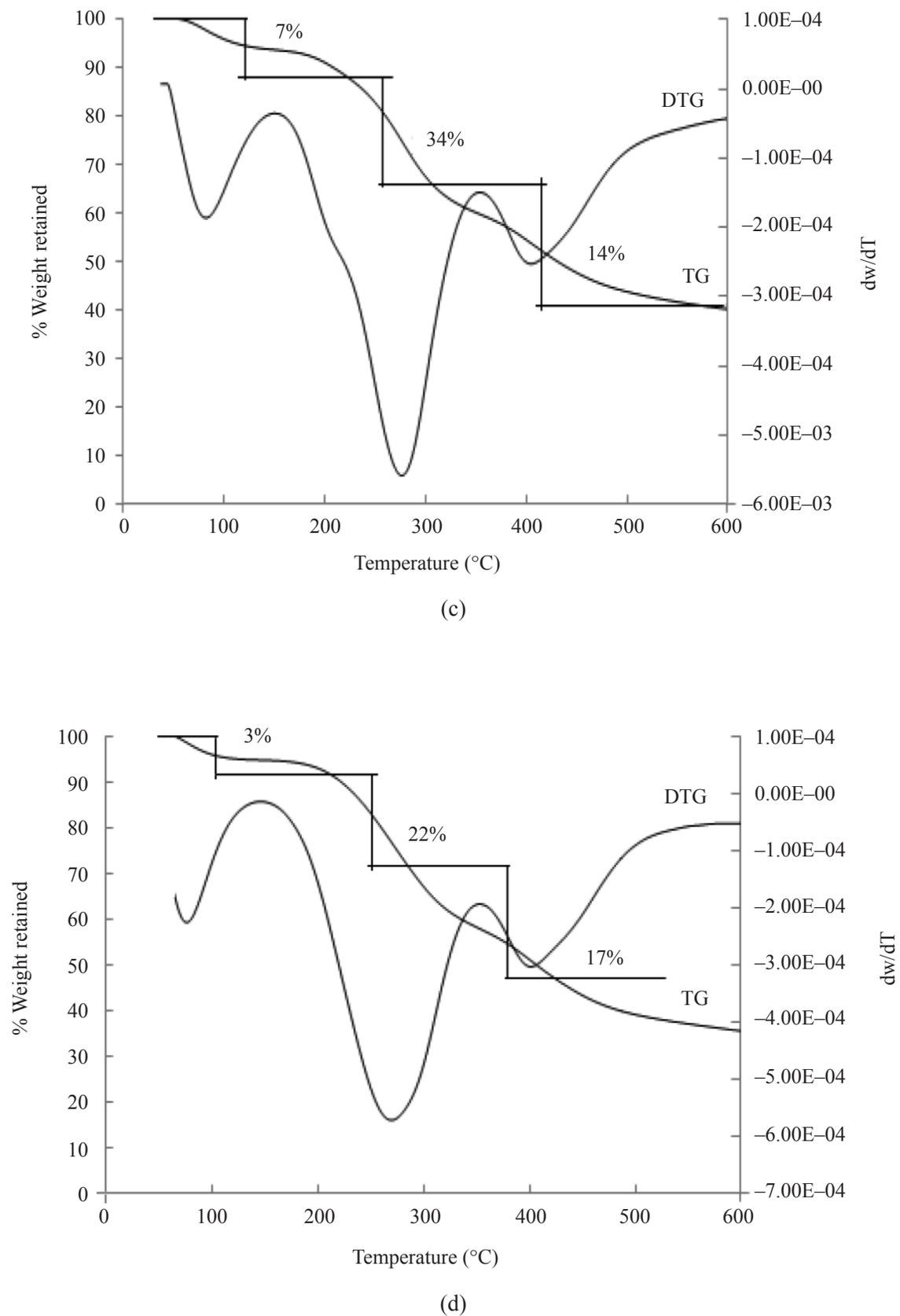
**Figure 3 (Cont.).** TG and DTA curves for (c) amidoxime-modified poly(AN-g-CS) and (d) homoPAN.
