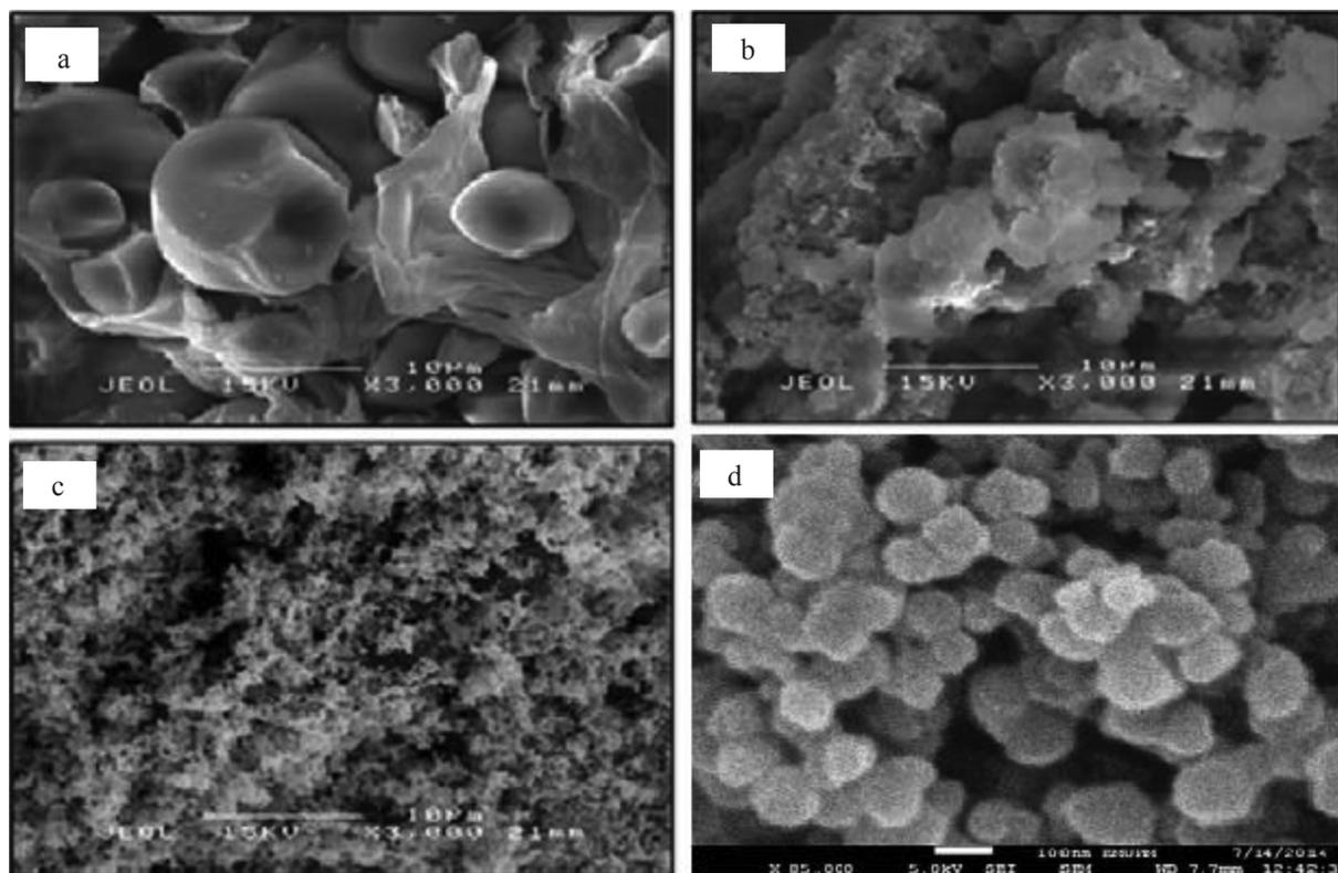
**Figure 2.** The SEM images of (a) CS (b) poly(AN-g-CS) (c) amidoxime-modified poly(AN-g-CS) and (d) homoPAN.
