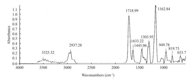
Figure 3. IR spectrum of the prepared ester product dimethacrylate.
