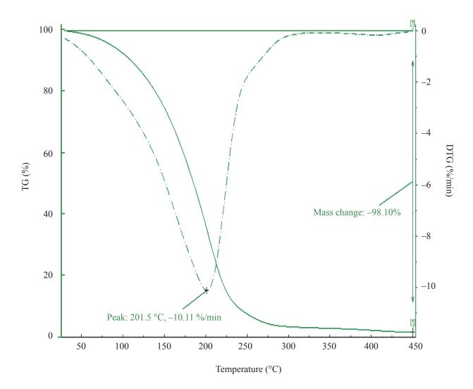
Figure 5. Thermal analysis diagram of the product ethylene glycol dimethacrylate.
