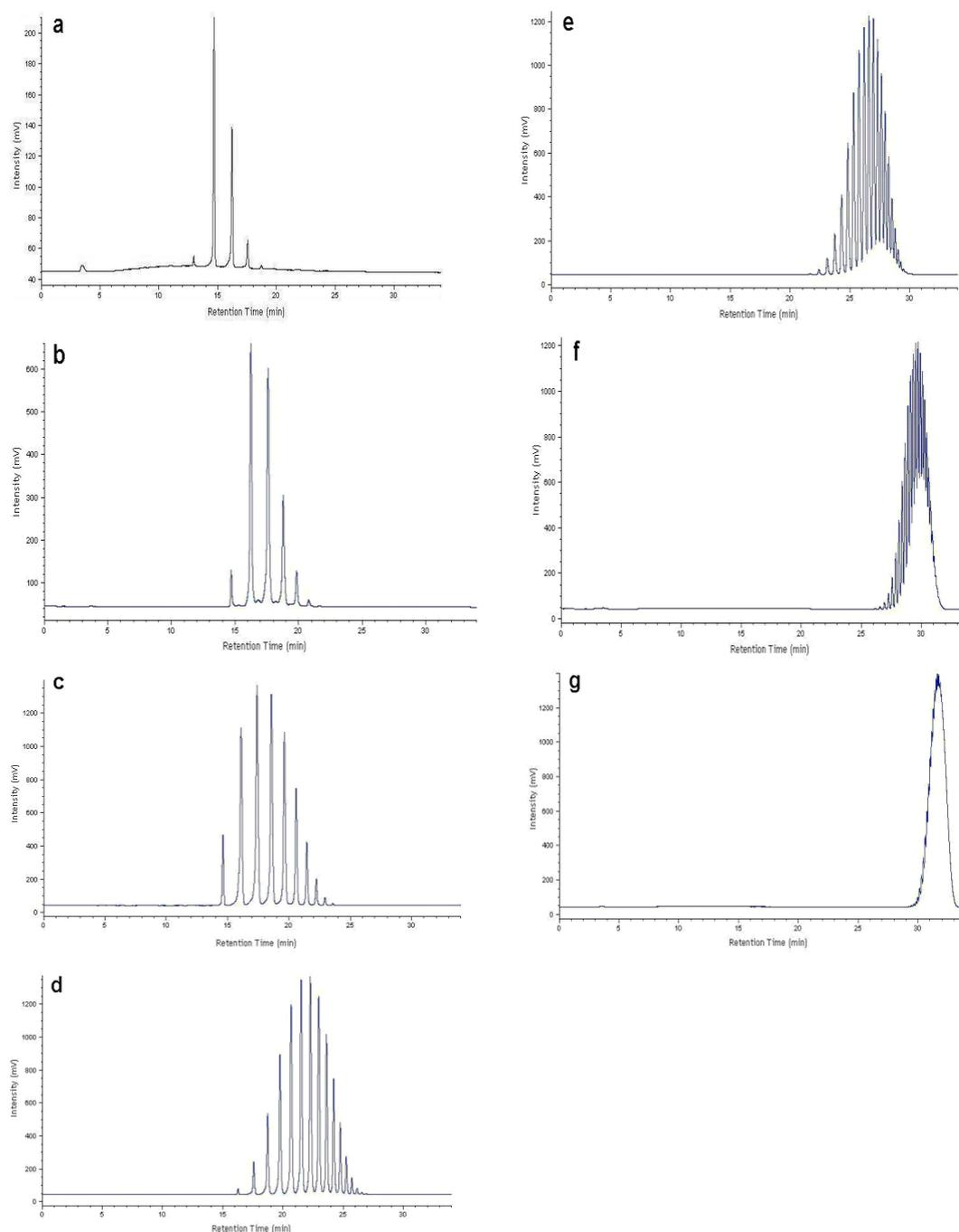
**Figure 1 :** Chromatograms of (a) PEG 200, (b) PEG 300, (c) PEG 400, (d) PEG 600, (e) PEG 1000, (f) PEG 1500 and (g) PEG 2000 using methanol as organic solvent. Conditions as described in the text.
