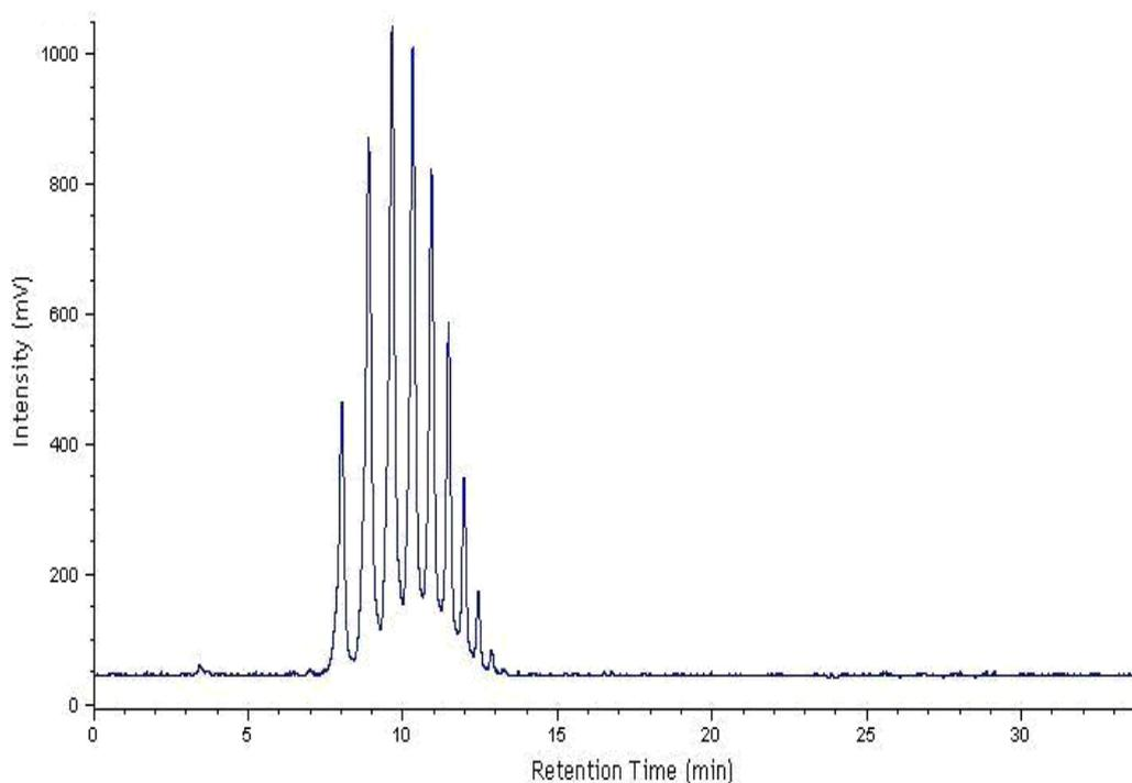
**Figure 2** : Chromatograms of PEG 400 using acetonitrile as organic solvent, instead of methanol. Conditions are described in the text.
