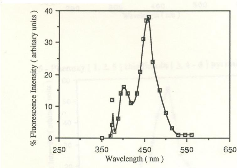
Figure 4: Fluorescence spectrum of 2-N-phenylalaninopurine ( $5.712 \times 10^{-4}$  M)
