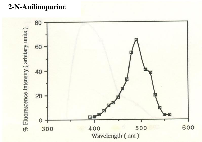
**Figure 2 :** Fluorescence spectrum of 2-N-anilinopurine ( $8.890 \times 10^{-4}$  M)
