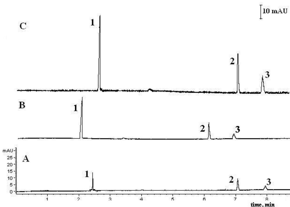
**Figure 2:** Separation of hydrophilic OPPs at mixture (A) 10 ppm, (B) 20 ppm and (C) 30 ppm for (1) dicotophos, (2) monocrotophos and (3) phosphamidon. Separation conditions remain the same as in Figure 1.
