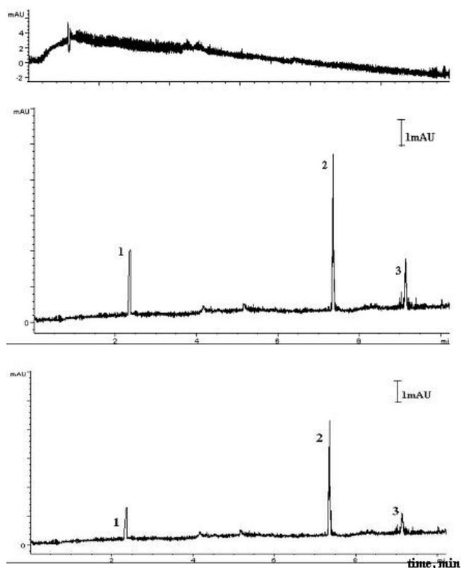
**Figure 3:** Electropherogram of extracted blank pond water (A) and of dicotophos (1), monocrotophos (2) and phosphamidon (3) at (B) 0.5 ppm and (C) 1 ppm which is the concentration after reconstituting to a final volume of 1 mL. Separation buffer contained 20 mM phosphate (pH 2.3), 10 mM SDS and 10% v/v methanol; applied potential -25kV; hydrodynamic sample injection for 50 s at 50 mbar.
