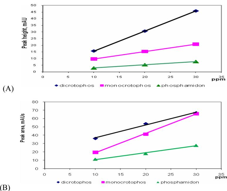
**Figure 1:** Calibration curves based on (A) peak height and (B) peak areas for the separation of hydrophilic OPPs in SRMM-MEKC. Separation buffer contained 20 mM phosphate (pH 2.3), 10 mM SDS and 10% v/v methanol; applied potential -25kV; hydrodynamic sample injection for 50 s at 50 mbar.
