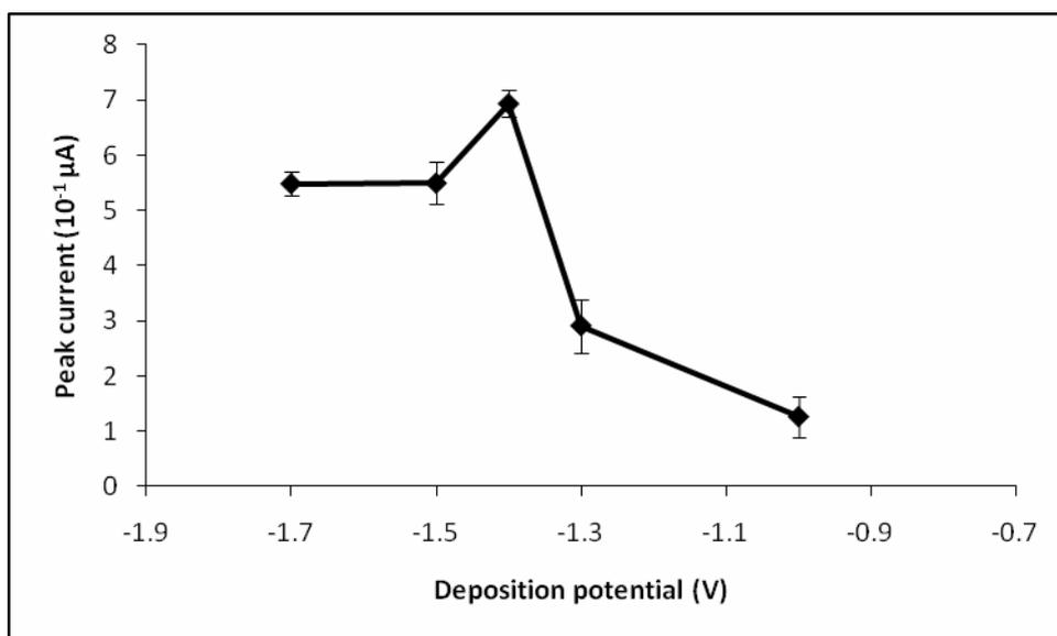
**Figure 5.** Effect of accumulation potential on the differential pulse stripping voltammetric peak of a Pb sensor in  $5 \text{ mgL}^{-1} \text{ Pb}^{2+}$ .
