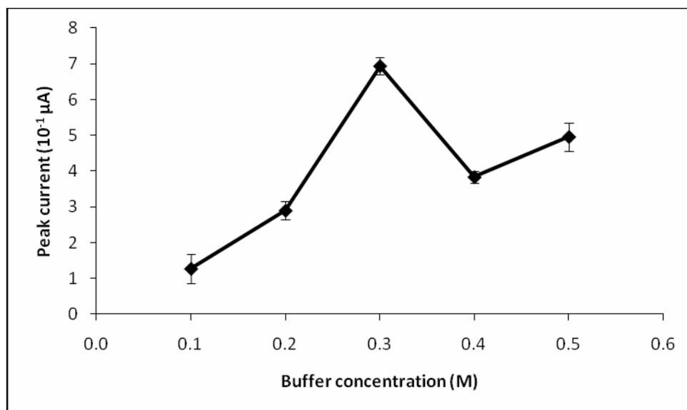
**Figure 3.** The effect of ammonia buffer concentrations on the differential pulse stripping voltammetric current of the Pb sensor in  $5 \text{ mgL}^{-1} \text{ Pb}^{2+}$ .
