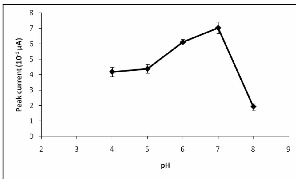
**Figure 2.** The effect of pH on the differential pulse stripping voltammetric peak current of a Pb sensor in  $5 \text{ mgL}^{-1} \text{ Pb}^{2+}$
