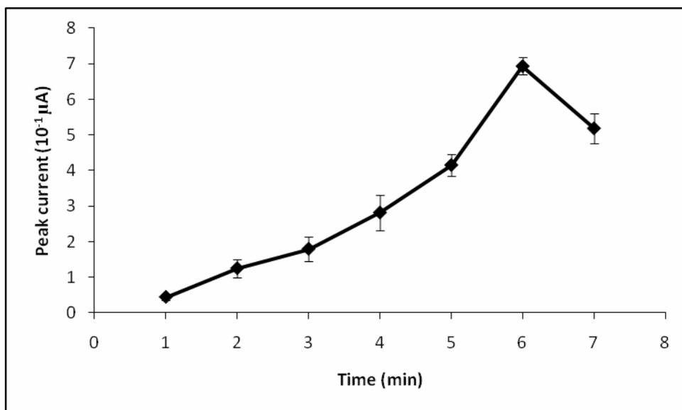
**Figure 4.** The effect of accumulation time on the differential pulse stripping voltammetric peak current of a Pb sensor in  $5 \text{ mgL}^{-1} \text{ Pb}^{2+}$ .
