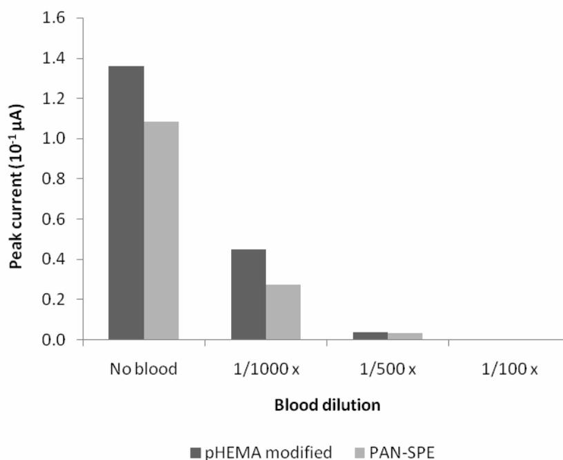
**Figure 7.** The effect on the lead sensor response when various volumes of blood serum was added to a buffer solution containing  $1 \text{ mg L}^{-1}$   $\text{Pb}^{2+}$  (1/1000x refers to 1 part of blood serum is diluted to 1000 times)
