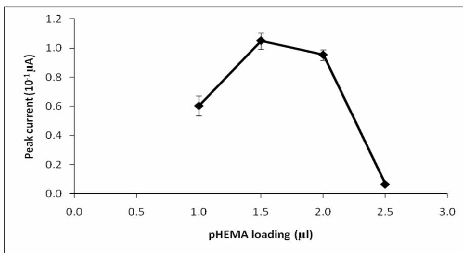
**Figure 1.** The effect of pHEMA loadings on the differential pulse stripping voltammetric peak current of a Pb sensor in  $5 \text{ mgL}^{-1}$   $\text{Pb}^{2+}$ . (1  $\mu\text{L}$  pHEMA = 1  $\mu\text{g}$ )
