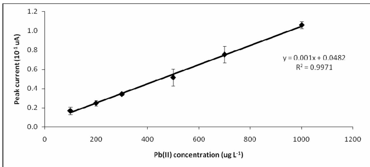
**Figure 6.** The calibration curve of the lead sensor for lead ion concentrations of 100 – 1000  $\mu\text{g L}^{-1}$   $\text{Pb}^{2+}$
