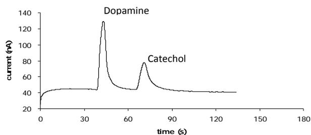
**Figure 2 :** Electropherogram of 250  $\mu\text{M}$  dopamine and catechol. Experimental conditions: detection potential, 0.8 V; separation voltage, 1300 V; pinched injection time, 20 s; running buffer, 20 mM MES (pH 7.0).
