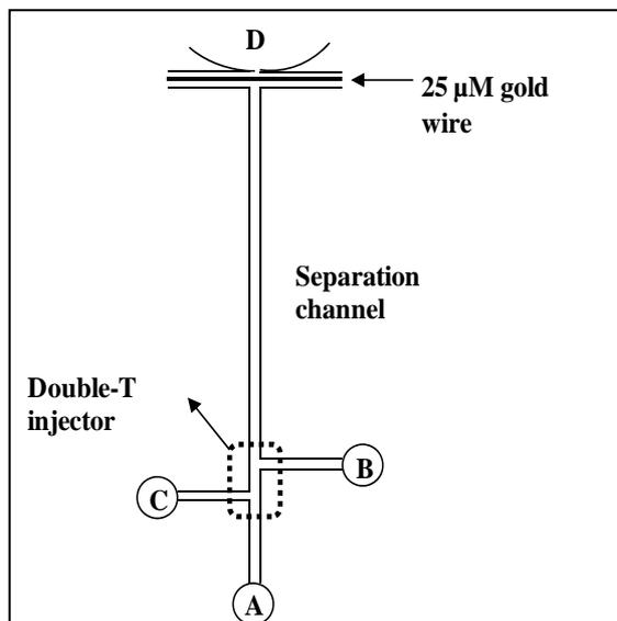
**Figure 1 :** Pattern of PDMS microchip (A) buffer reservoir, (B) sample reservoir, (C) sample waste reservoir and, (D) waste reservoir. Channels: 50  $\mu\text{m}$  width, 50  $\mu\text{m}$  depth. Separation channel: 52 mm length. Double-T injection channel: 100  $\mu\text{m}$  length.
