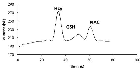
**Figure 3 :** Electropherogram of 250  $\mu\text{M}$  Homocysteine, glutathione and N-acetyl-L-cysteine. Experimental conditions: detection potential, 0.7 V; separation voltage, 1300 V; pinched injection time, 20 s; running buffer, 20 mM boric acid (pH 8.5).
