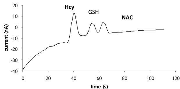
**Figure 4:** Electropherogram of 150  $\mu$ M Homocysteine, 200  $\mu$ M glutathione and 200  $\mu$ M N-acetyl-L-cysteine. Experimental conditions: detection potential, 1.0 V; separation voltage, 1300 V; pinched injection time, 20 s; running buffer, 20 mM MES and 1 mM SDS (pH 6.0).
