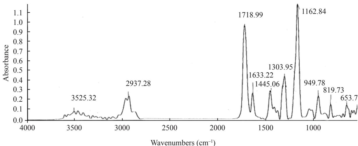
**Figure 3.** IR spectrum of the prepared ester product dimethacrylate.
